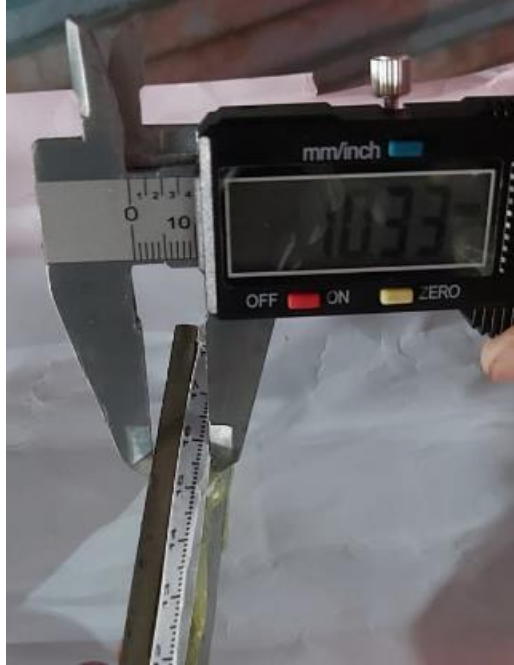
Figure 3-5: Overall thickness of Double Cantilever Beam joint
