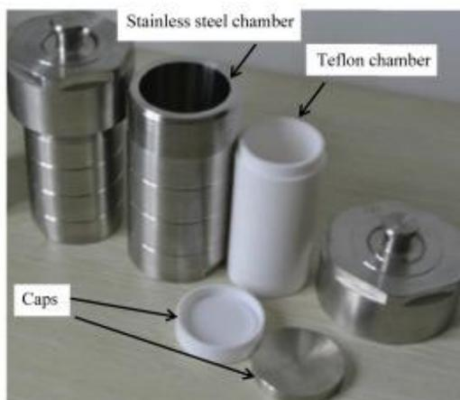
Figure 18 Autoclave used for the hydrothermal synthesis technique.
