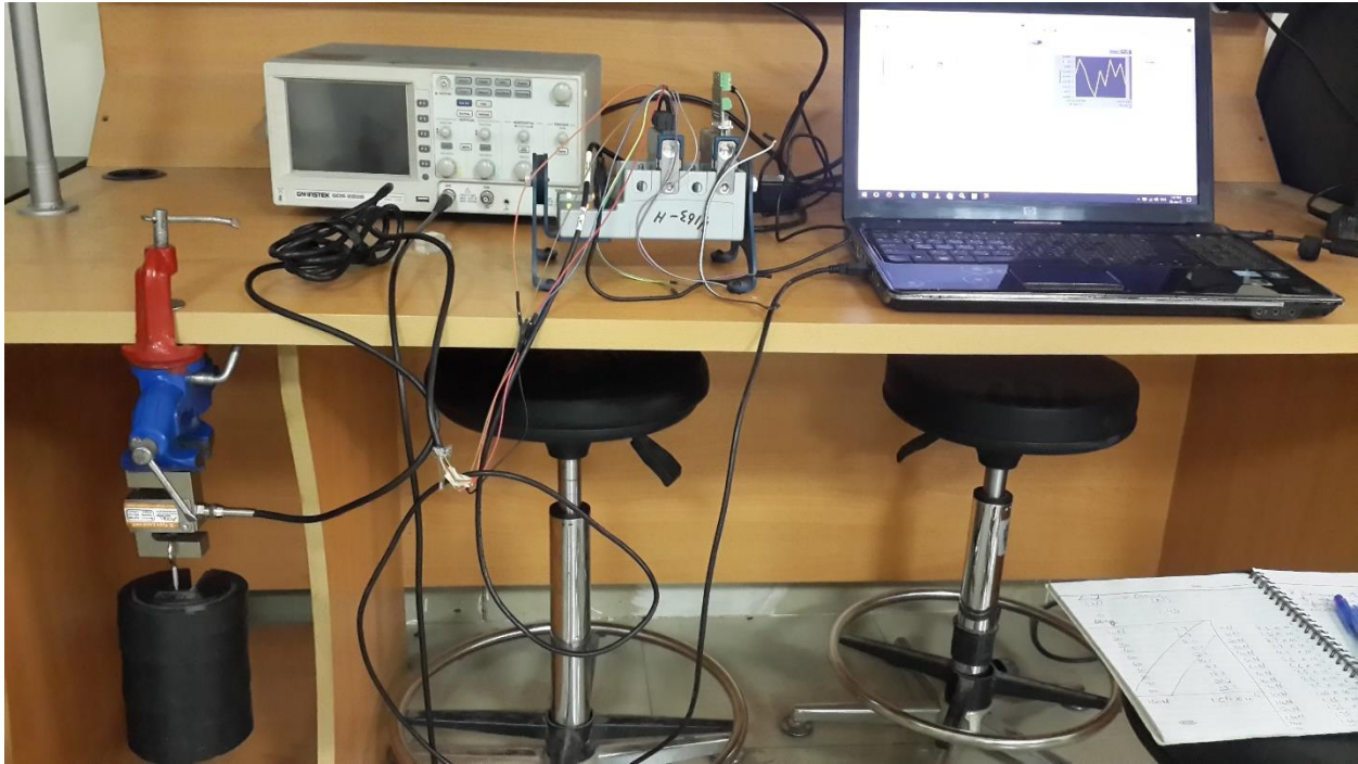
Fig. 11 Setup for calibration of Load Cell
