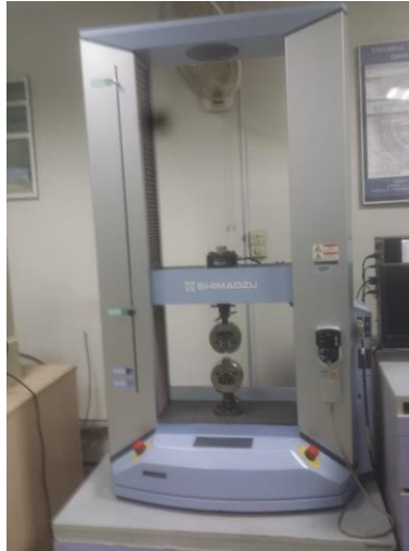
Figure 3-12: Universal Testing Machine (SHIMADZU) with 20 kN Load cell
