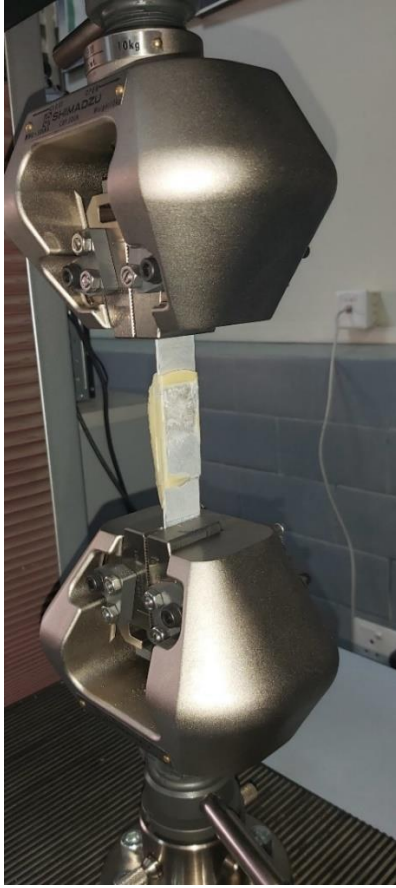
Figure 3-13: Specimen under Tensile shear testing (UTM, 100 kN load cell)
