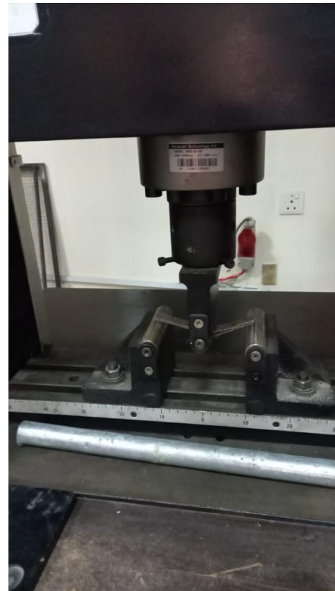
Figure 3.13 Flexural test (specimen breakage) on UTM
