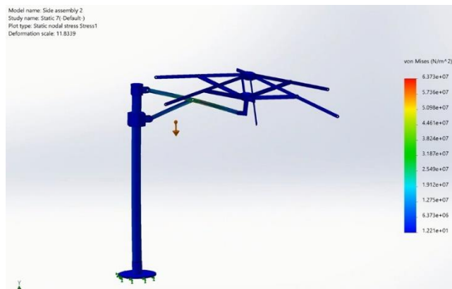
Figure 38 Von Mises – Open Position
