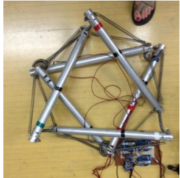
Figure 8: Collapsing into the star elongation shape. [3]
