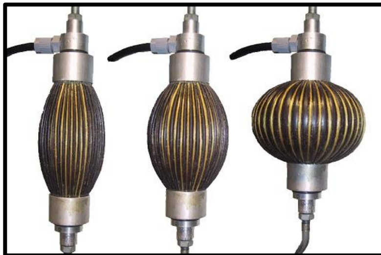
Figure 12: McKibben Actuators in their rest state and under pressure (left to right) [32]
