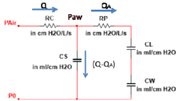
Figure 16. Equivalent electrical model of lung.
