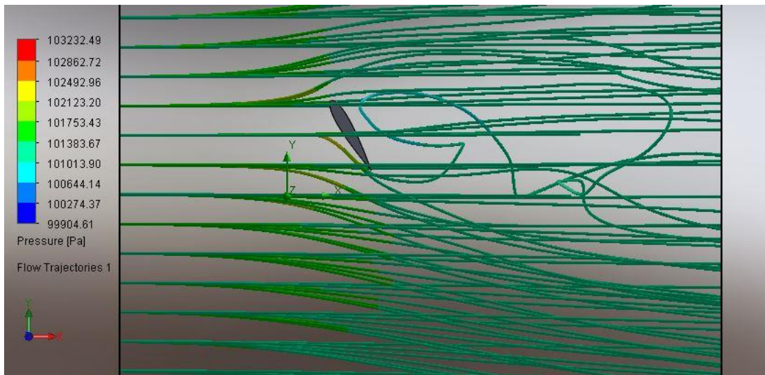
Figure 31: Hydrofoil Under Water Flow (60° AOA)
