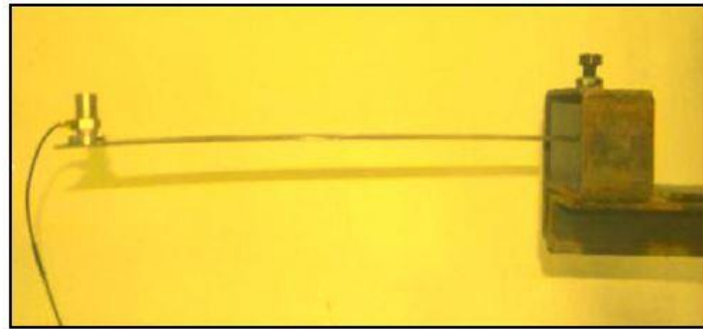
Figure 3.7: Experimental setup of a fixed free beam with an accelerometer mounted at the free end [12]
