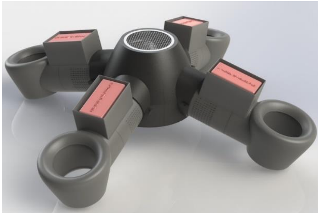
Figure 12: Proposed Bladeless Penta-copter
