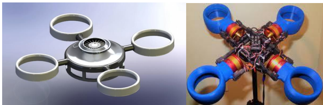
Figure 7: Bladeless Drone with central propulsion (taken from [23]) and Independent Propulsion (taken from [27])
