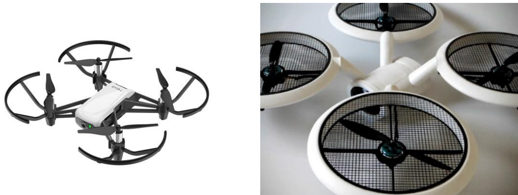
Figure 3: Drone Propeller Guards - Partially (taken from [20]) and Fully (taken from [21]) Surrounded
