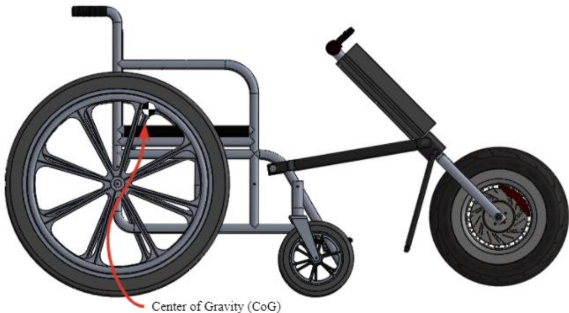
Figure 22: Location of Center of Gravity of the System (80 kg added for user)
