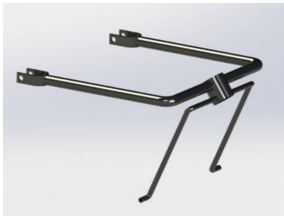
Figure 20: Chassis Part which Connects to the Wheelchair
