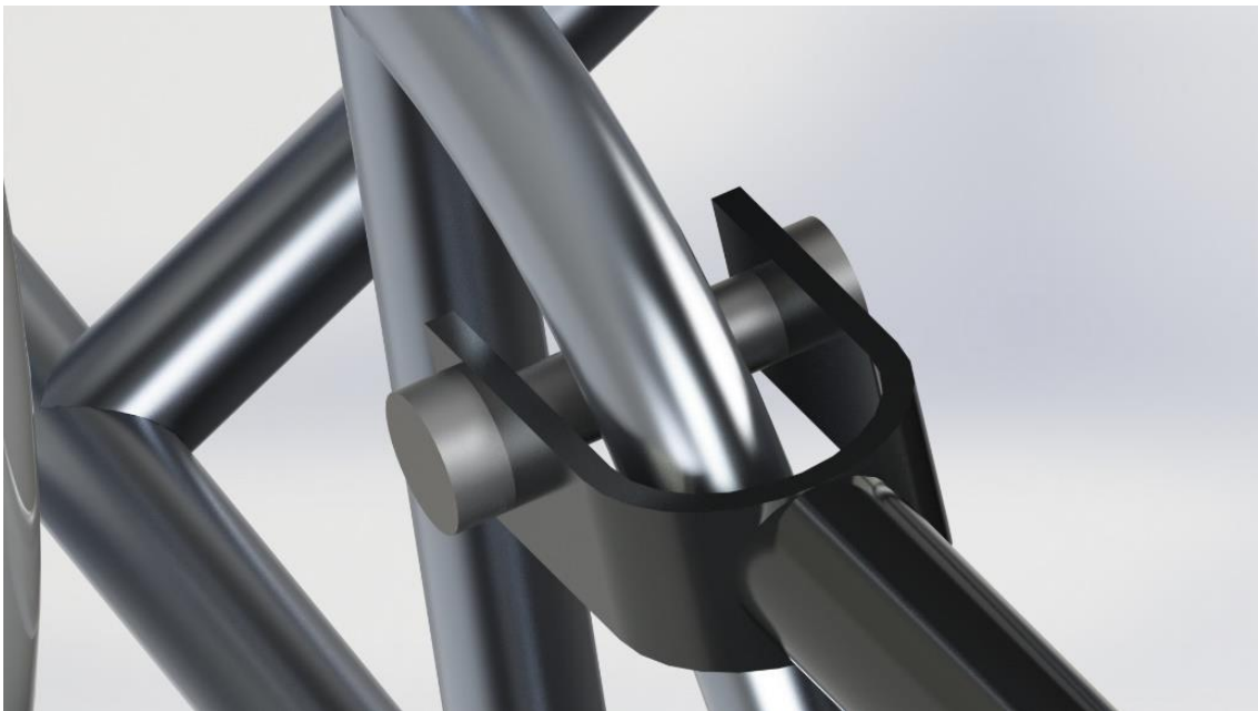
Figure 21: Chassis Connected to the Wheelchair by dint of a Bolt and Nut
