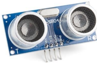
Figure 8 HC-SR04 Position Sensor
