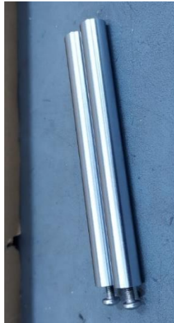
Figure 26: Fabricated Guide Rods
