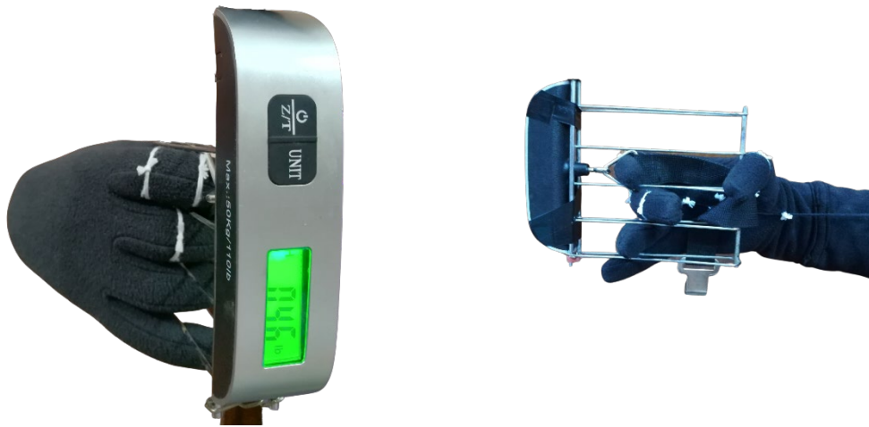
Figure 4-5: force measurement using a modified weight scale to act as a grip strength dynamometer
