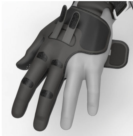
Figure 1-1: A soft glove used for forced Flexion and Extension of three fingers required for object gripping.
