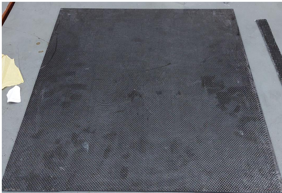
Figure 4 Sample Plate 450x450mm
