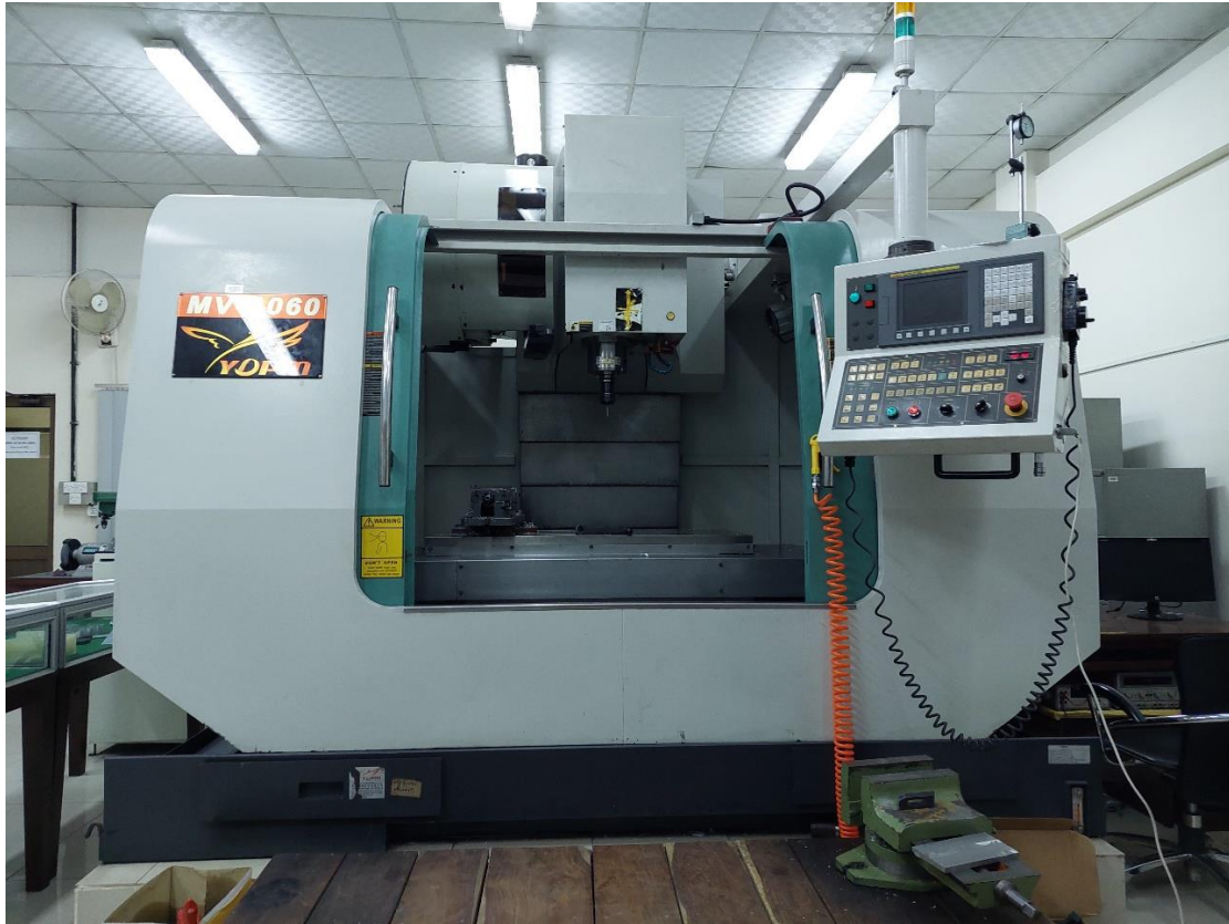
Figure 6 CNC milling machine MV-1060
