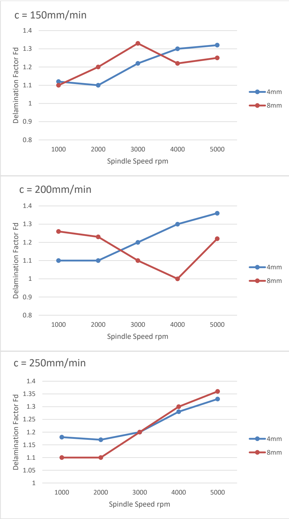
Figure 17 Effect of drilling parameters on delamination
