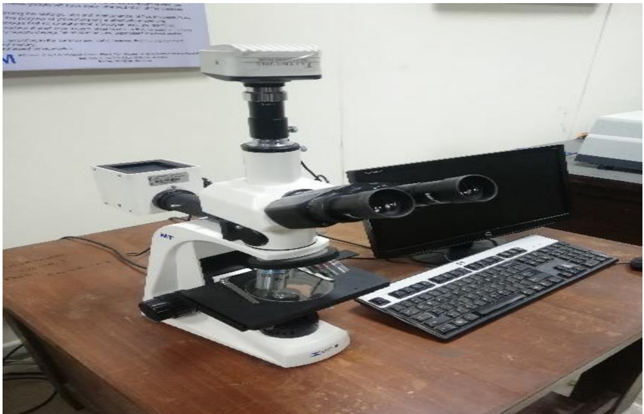
Figure 26 Optical Microscope to analyze tool wear of cutting inserts
