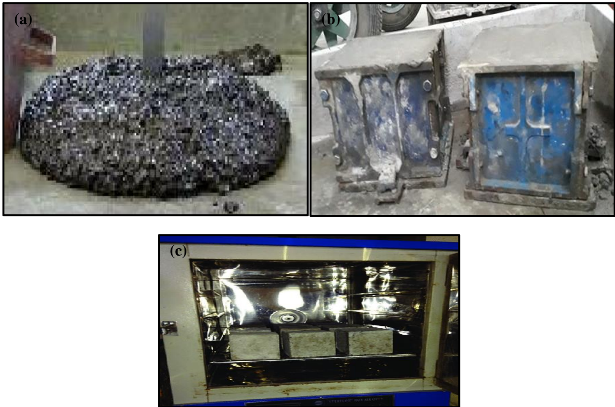
Figure 3.5. Geopolymer concrete (a) Green concrete (b) Casting of cubes (c) Temperature curing
