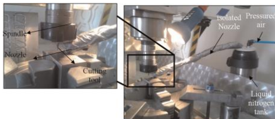
Figure 8 (Experimental setup using cryogenic cooling) [22]
