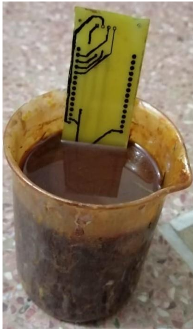
Figure 16 Circuit reaction with Ferric Chloride
