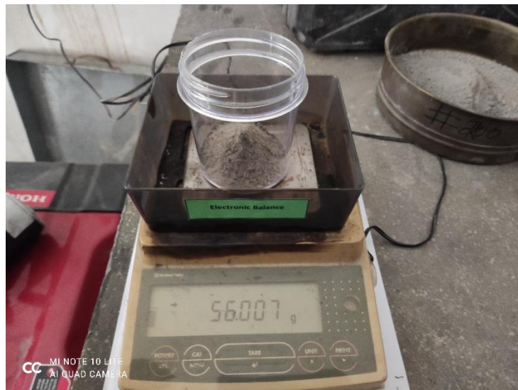
Figure 3.4: Weighing the dry material.
