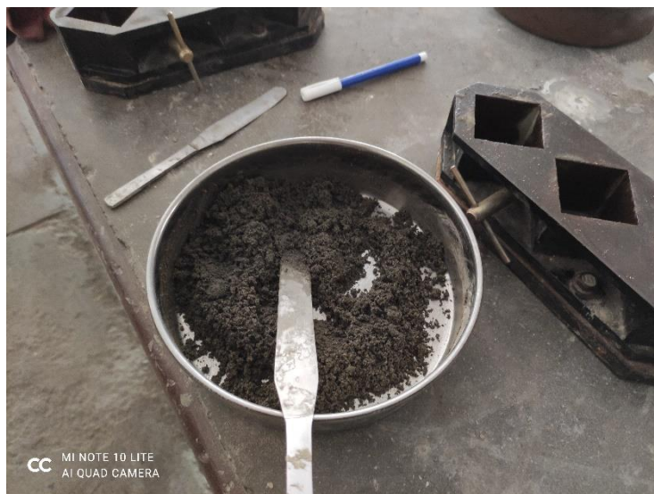
Figure 3.6: Preparation of Cement Mortar
