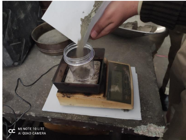
Figure 3.3: Weighing the dry material.
