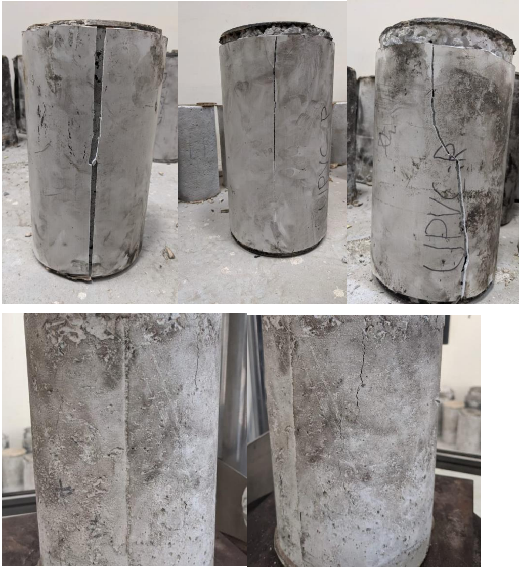
Figure 22: UPVC confined specimens failure
