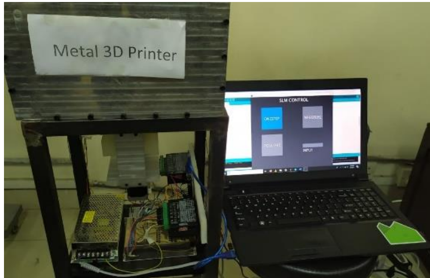
Figure 21 SLM Metal 3D Printer with GUI control
