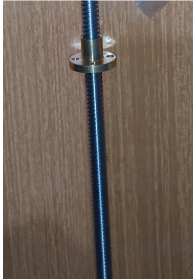
Figure 11 Lead screw (2mm pitch)(8mm dia) with the brass nut
