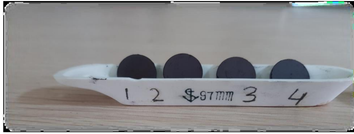
Fig 2.2 pellets of ferrites [38]
