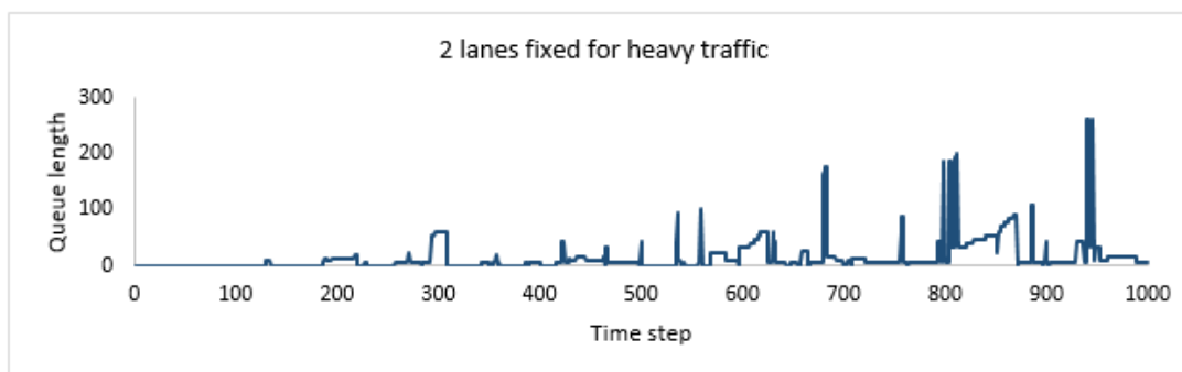
FIGURE 4.7: Configuration of 2 lanes fixed for heavy traffic as vehicular input in Actuated traffic light control
