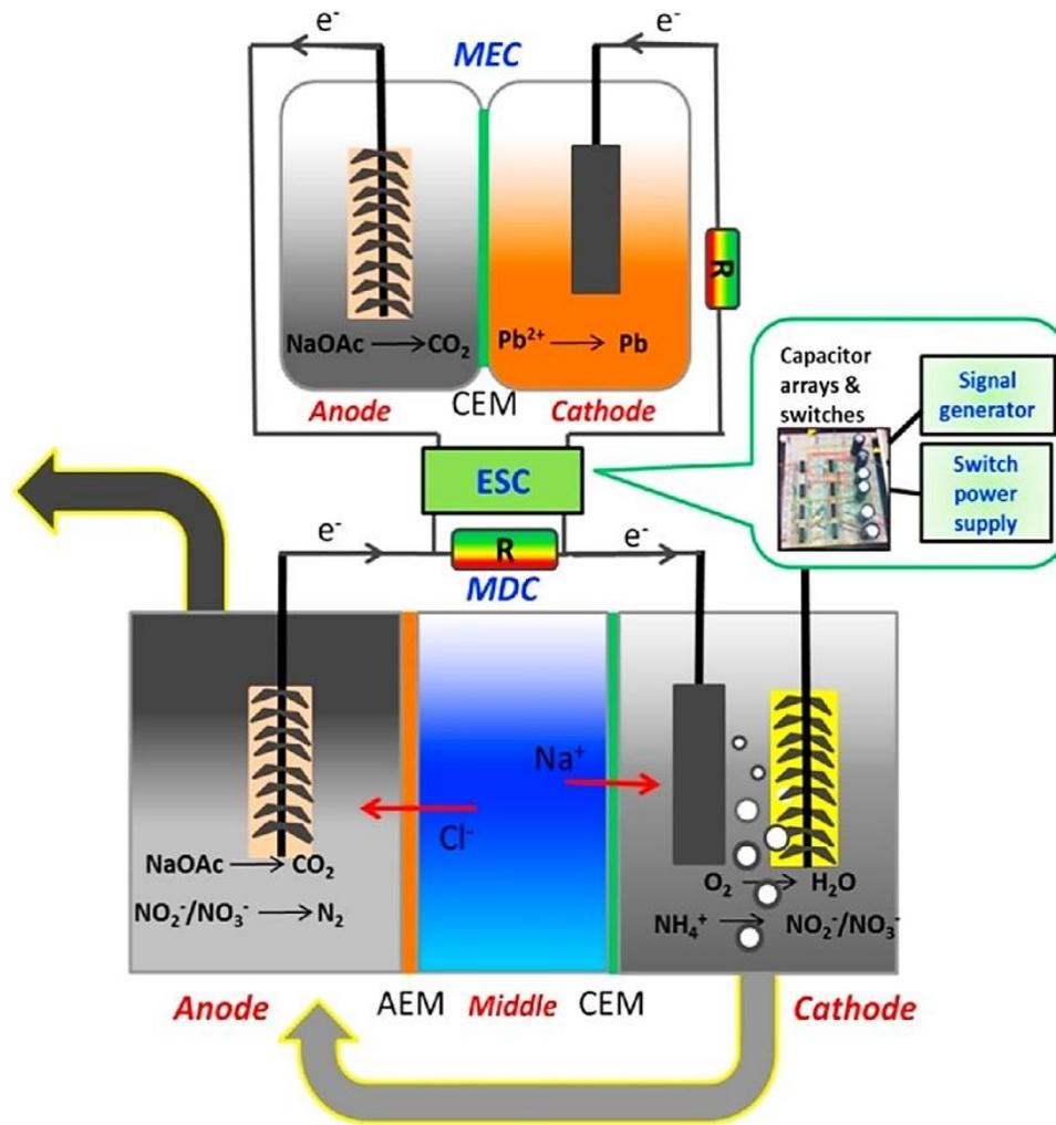
Figure 2-7 : Microbial Desalination Cell (MDC)- Microbial Fuel Cell (MEC) Hybrid System[66]
