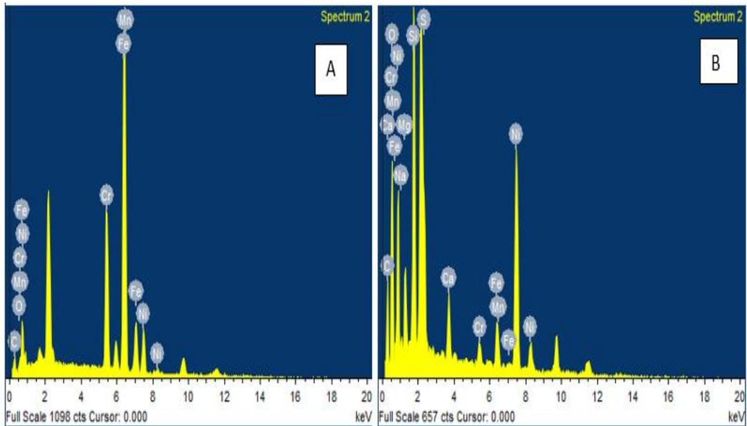
Figure 4-10 : EDS results of Stainless steel mesh 304L cathode (a) before use (b) after use.
