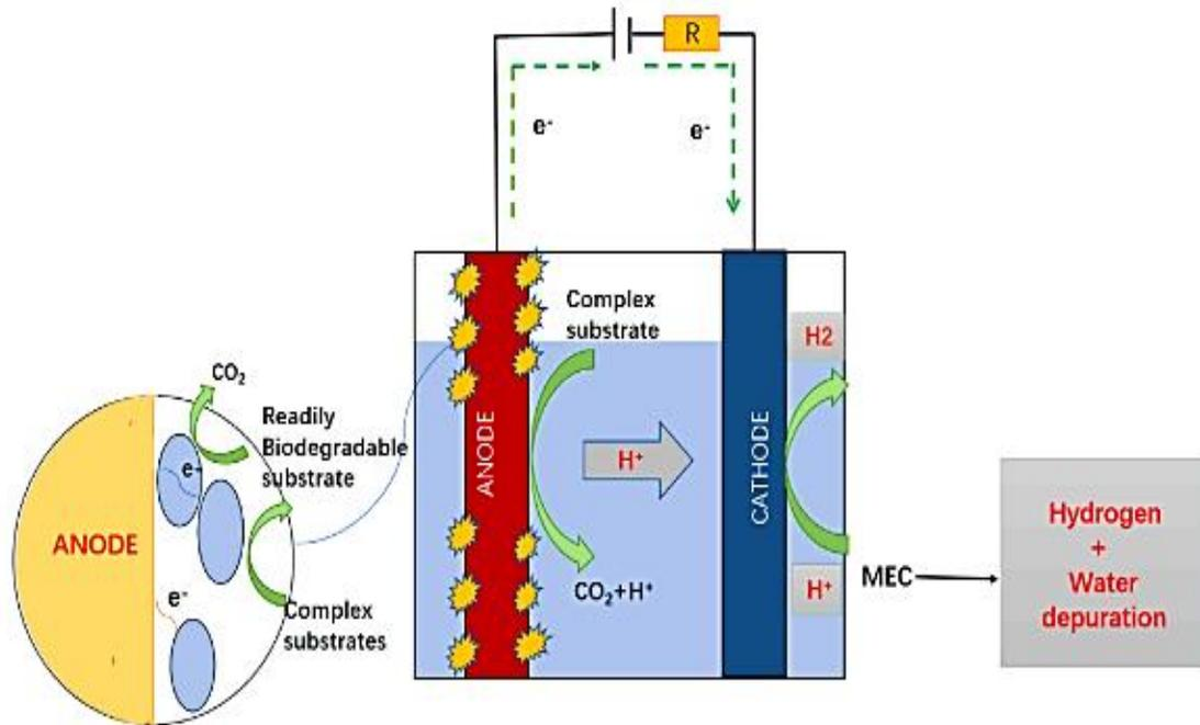
Figure 2-3 : Single Chamber Microbial Electrolysis Cell [12]
