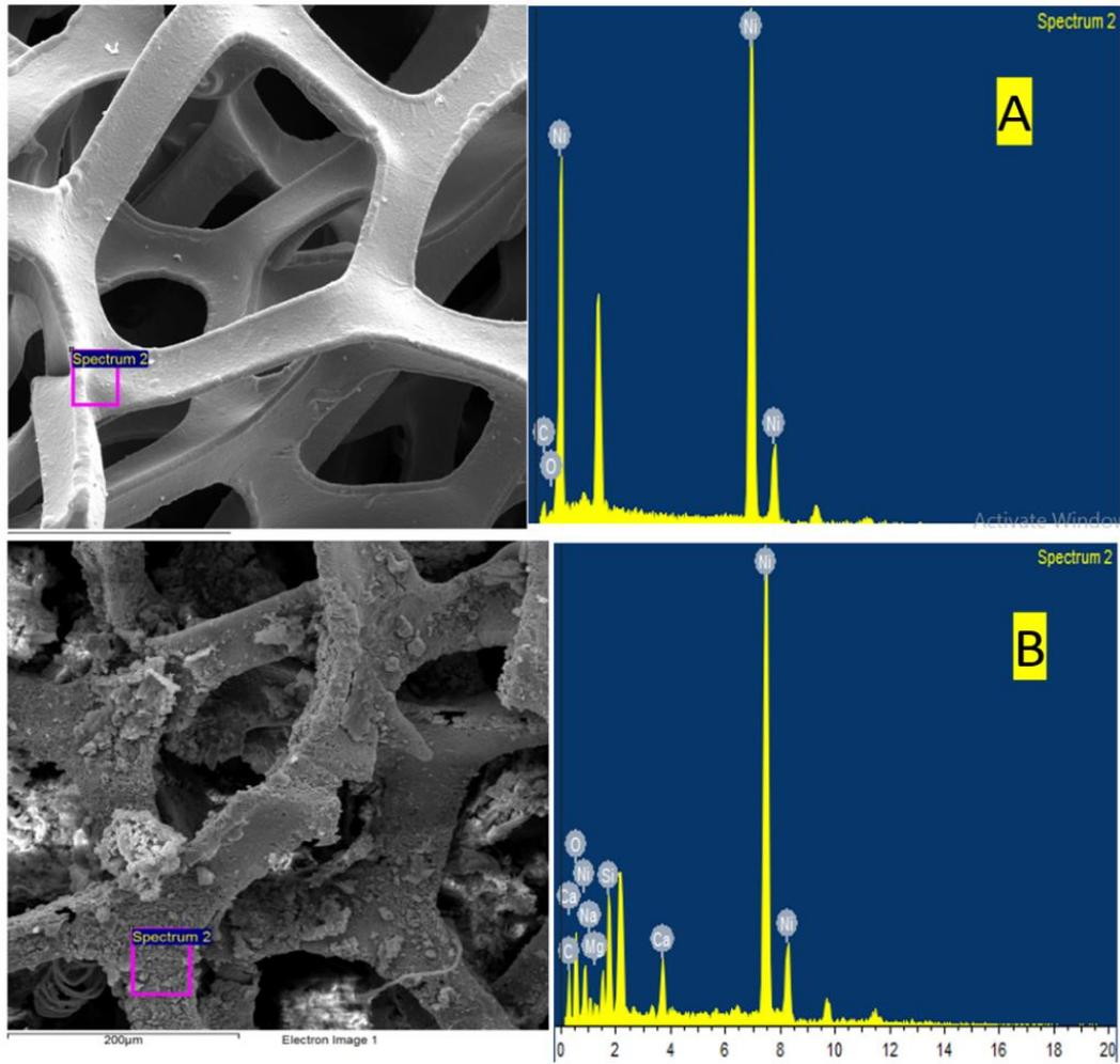
Figure 4-7 : EDS results of Ni-foam anode (a)before use and (b) after use
