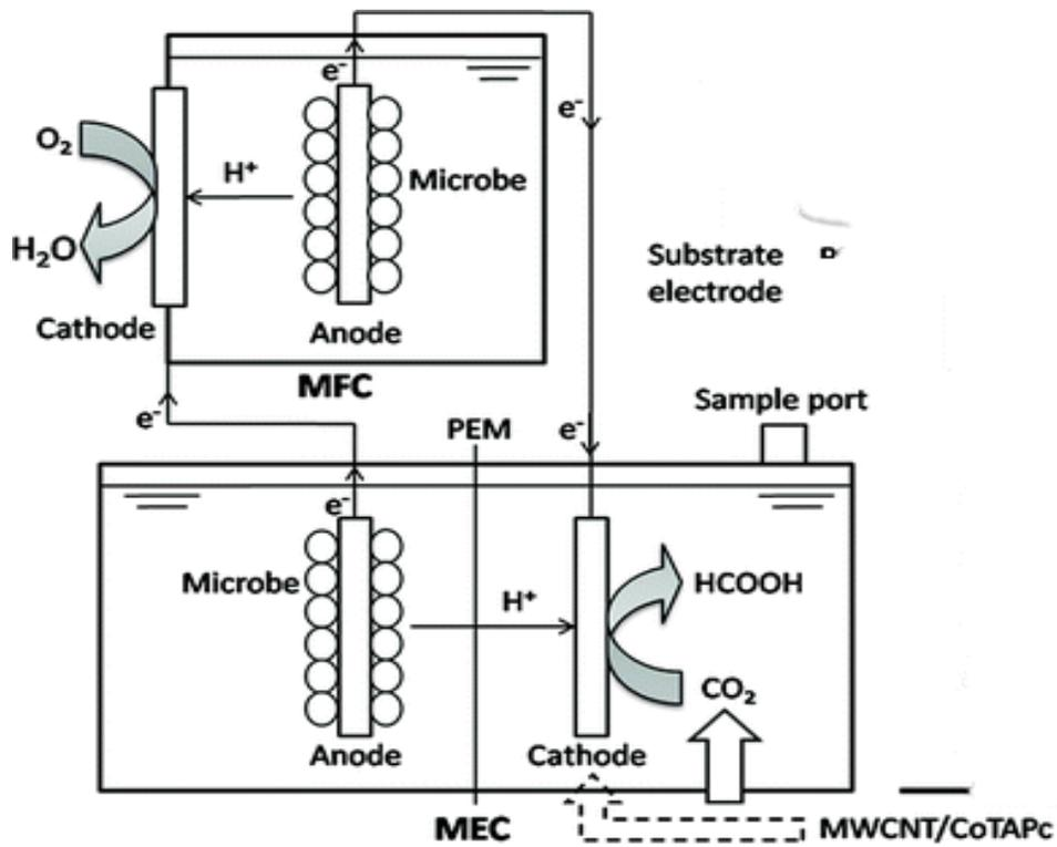
Figure 2-5 : Microbial Electrolysis Cell (MEC) - Microbial Fuel Cell (MFC) Hybrid System [59]
