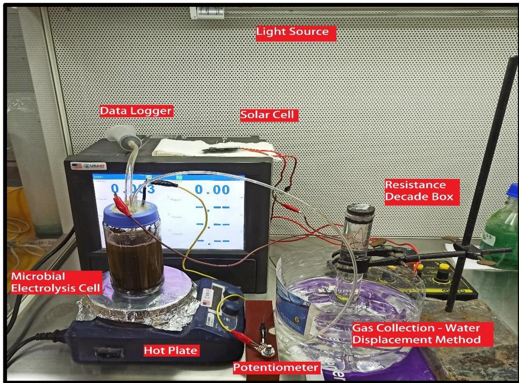
Figure 3-8 : Set-up of complete lab-scale MEC system
