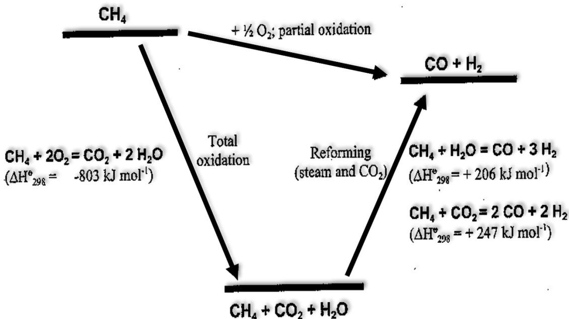
Figure 1-3 : Thermodynamic representation of the partial oxidation and steam reforming of methane [15]
