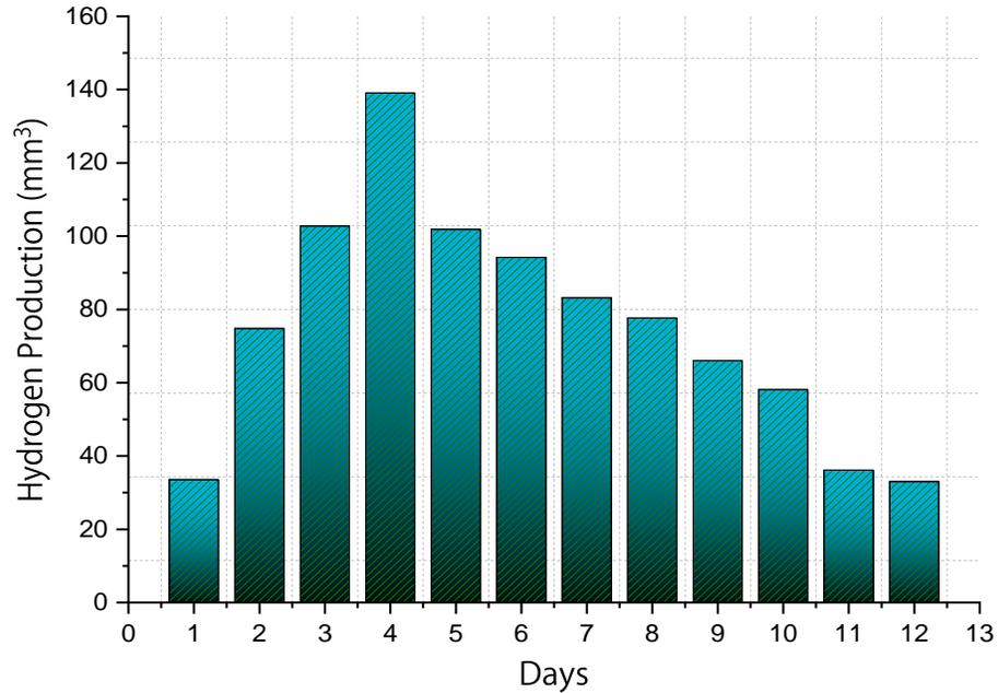
**Figure 4-2 : Hydrogen production using rate limited bio-anode - Microbial Electrolysis Cell**
