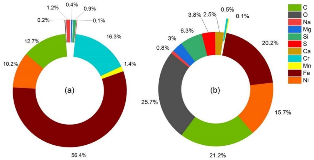
Figure 4-11: Elemental compositions (weight %) of Stainless-steel mesh 304L (a) before and (b) after experimentation
