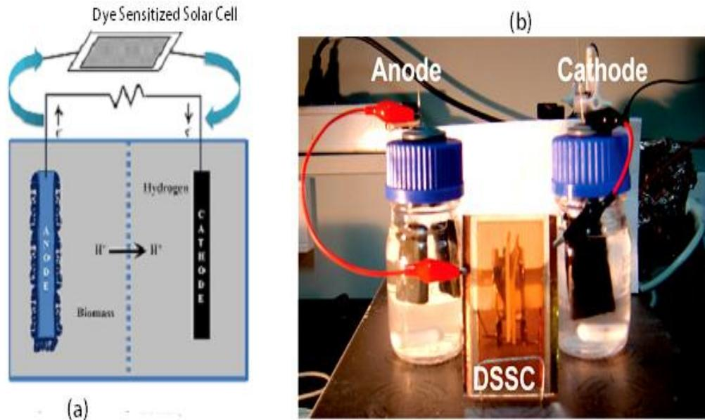
**Figure 2-6 : (a) Schematic diagram of self-sustained Hybrid system - Microbial Electrolysis Cell (MEC) - Dye Synthesized Solar Cell (DSSC). (b) Experimental setup of Microbial Electrolysis Cell (MEC) - Dye Synthesized Solar Cell (DSSC) Hybrid system [62][63]**
