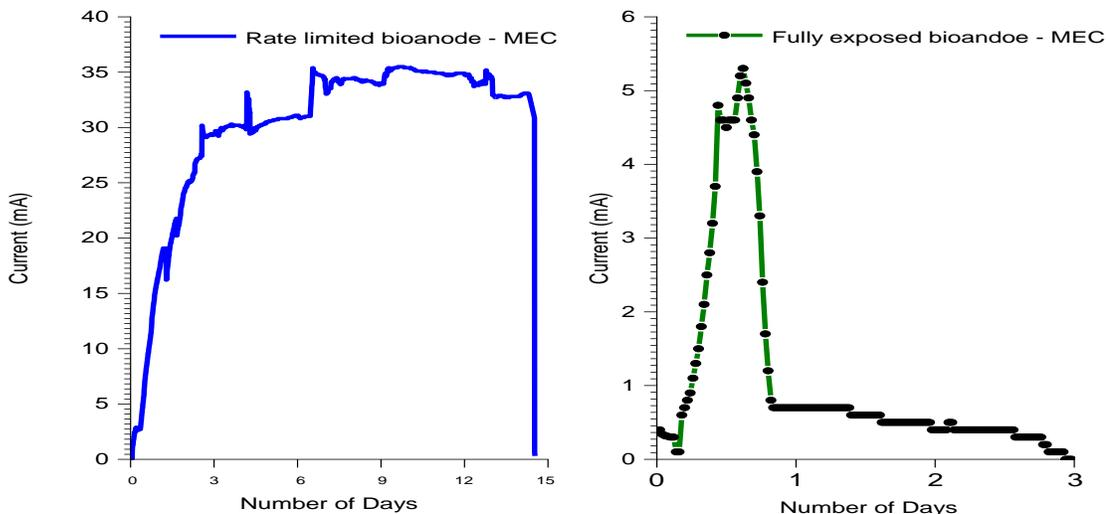
**Figure 4-5: Current produced in Rate limited bio-anode - MEC (left) and fully exposed bio-anode - MEC (right)**
