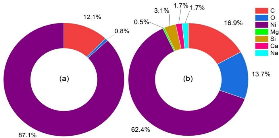
**Figure 4-8 Elemental compositions (weight %) of Ni-foam anode (a) before and (b) after experimentation**
