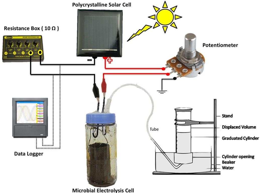
Figure 3-6 : Schematic representation of the complete MEC system
