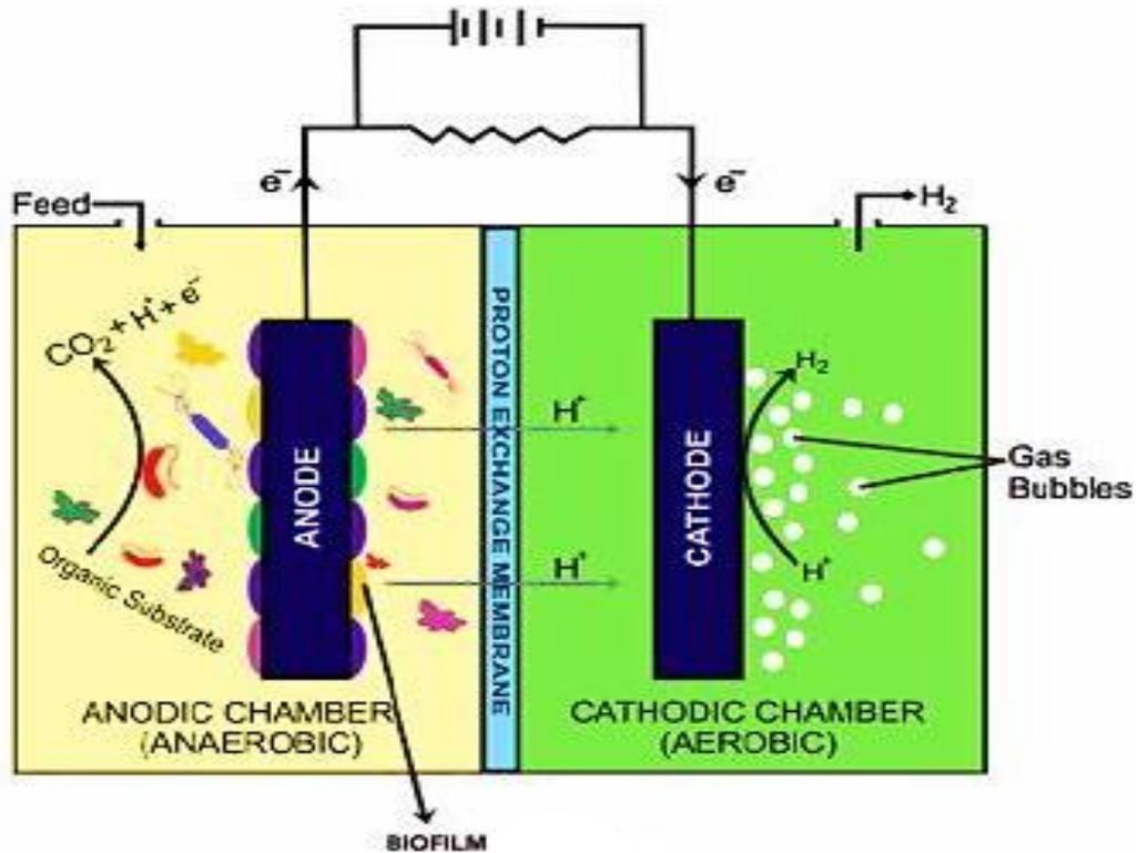
Figure 2-2 : Double Chamber Microbial Electrolysis Cell [13]
