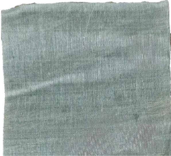
**Figure 3-4 : Stainless steel mesh grade 304L - cathode**
