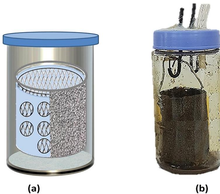
Figure 3-2 : (a) Schematic and (b) Experimental representation of the MEC Design
