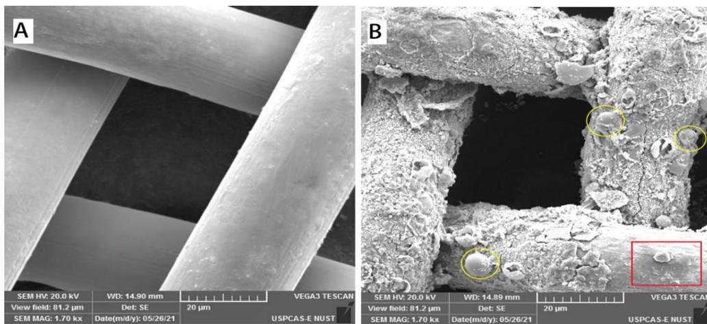
**Figure 4-9: Scanning Electron Microscopy (SEM) images of Stainless Steel Mesh 304L cathode with 20um magnification (A) before utilization and (B) after use (Round or circular microbial community was marked with yellow circles and debris-free SSM wire was marked with red rectangular box )**
