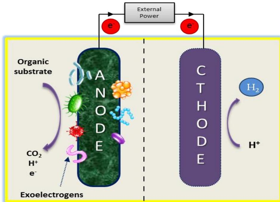
Figure 2-1 : Microbial Electrolysis Cell (MEC) - schematic diagram
