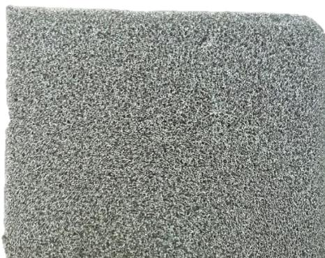
Figure 3-3 : Ni-foam with 300g/m<sup>2</sup> surface density - anode
