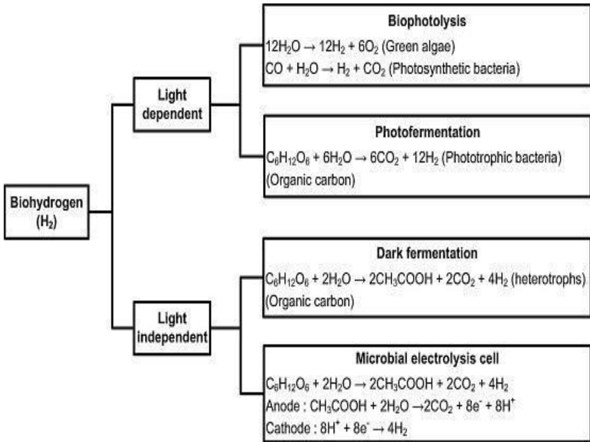
Figure 1-5 : Biological ways for producing biohydrogen (H<sub>2</sub>) [20]
