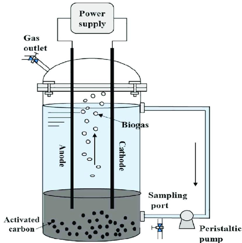
Figure 2-4 : Schematic diagram of the Microbial Electrolysis Cell (MEC) - Anaerobic Digestion (AD) [57]
