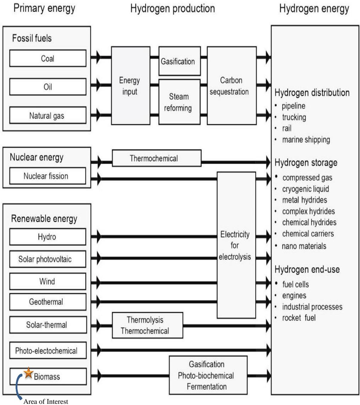
Figure 1-2 : Hydrogen energy production methods and major uses of hydrogen gas [13]
