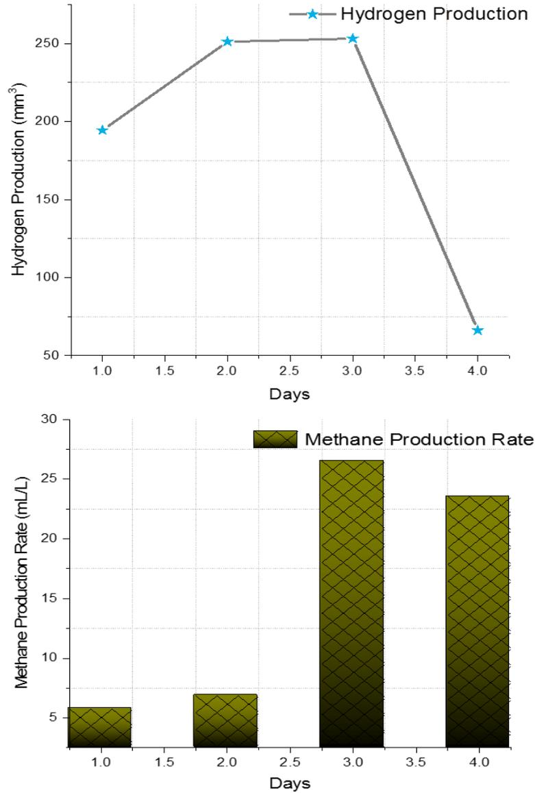
**Figure 4-4: Bioenergy production Trends using fully exposed Microbial Electrolysis Cell (above) hydrogen production (below) Methane Production rate**
