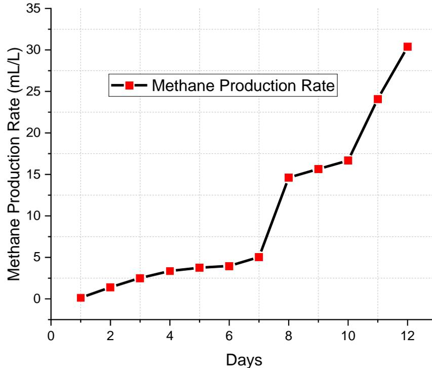
Figure 4-3 : : Methane production rate using rate limited bio-anode - Microbial Electrolysis Cell
