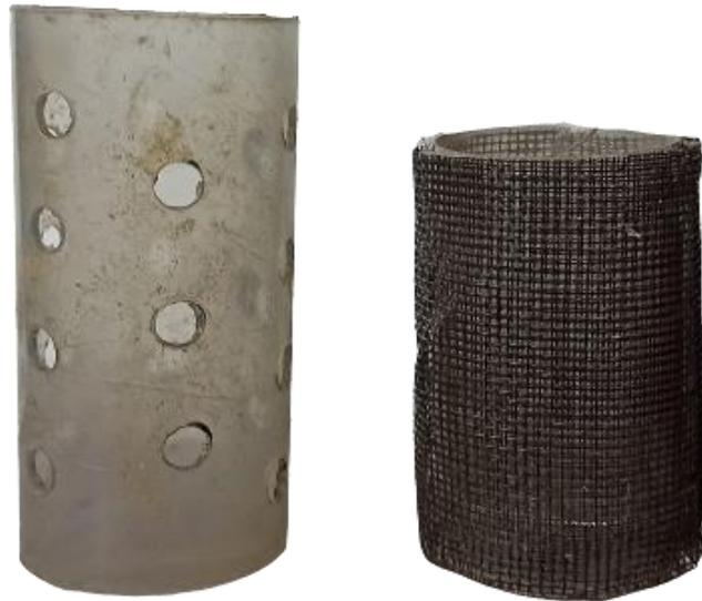
**Figure 3-5 : Rate limited bio-anode - MEC (left) and fully exposed bio-anode - MEC (right)**
