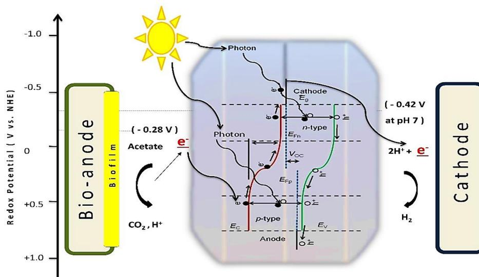
Figure 4-1 : Solar - MEC system electron transfer mechanism representing Z scheme of photosynthesis
