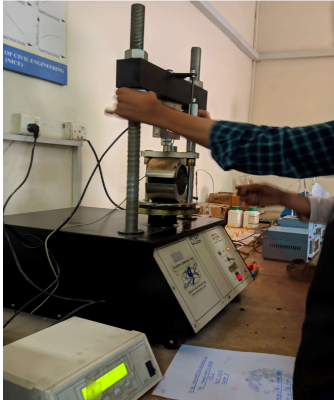
Figure 3.16 Marshall Stability and Flow Test
