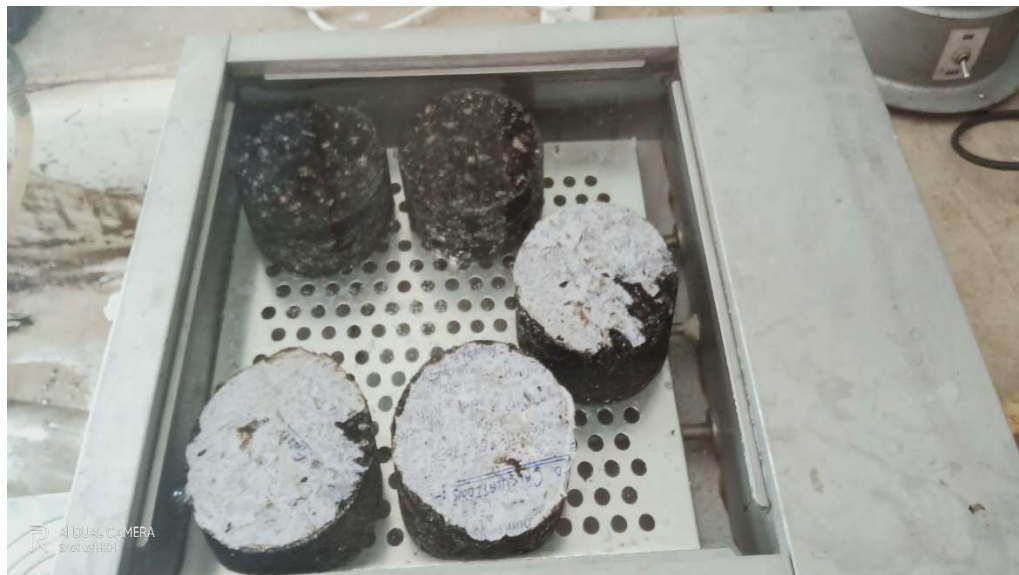
Figure 3.15 Marshall Samples being placed in water bath.
