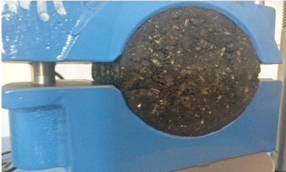
Figure 2.6 Marshall Stability Test
