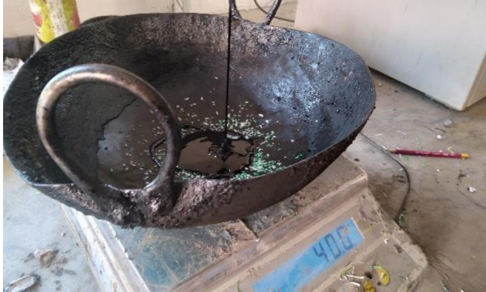
Figure 3.10 Mixing Bitumen with crushed PET bottles
