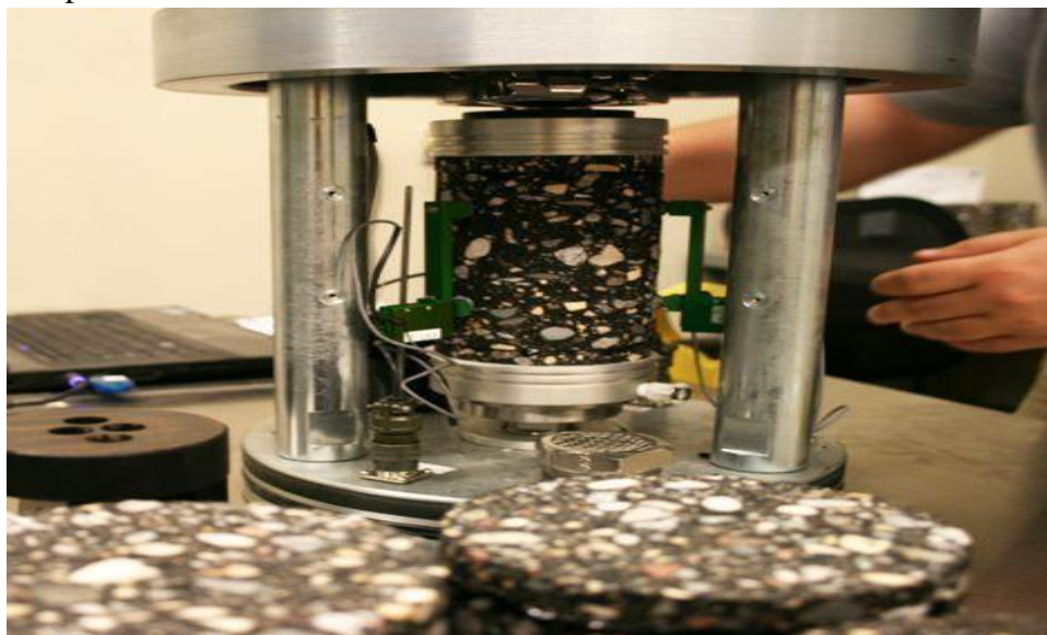
Figure 2.5 Triaxial Testing of Asphalt Cake
