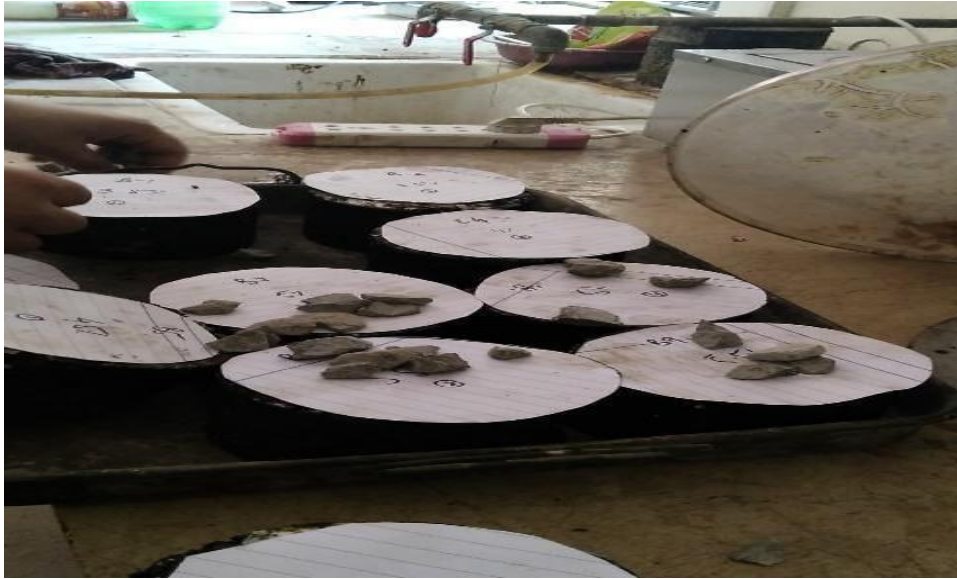
Figure 3.6 Prepared Asphalt Concrete Cakes
