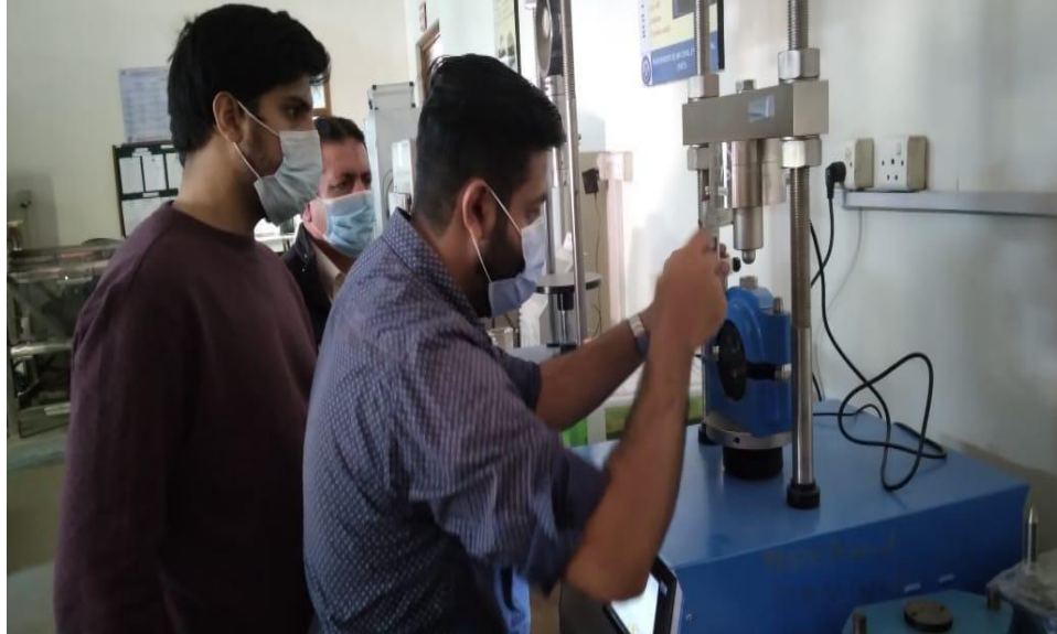
Figure 3.8 Stability and Flow Test
