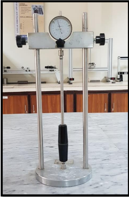
FIGURE 3-4 LENGTH COMPARATOR CALIBRATION FIGURE 3-5 SAMPLE TESTING ON LENGTH COMPARATOR
