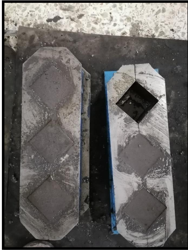
FIGURE 3-6 CUBES FOR COMPRESSION TESTING
