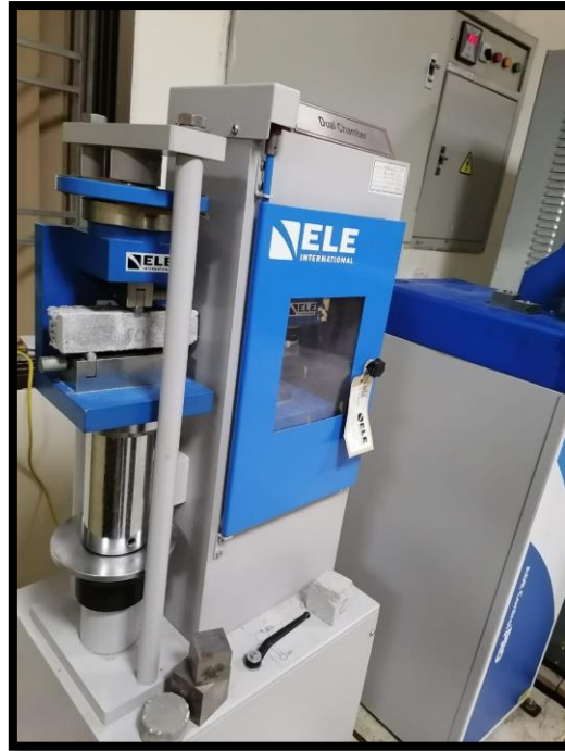
FIGURE 3-9 COMPRESSION AND FLEXURE TESTING MACHINE
