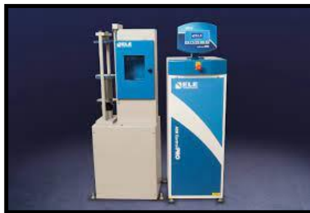
FIGURE 3-7 COMPRESSION AND FLEXURE TESTING MACHINE
