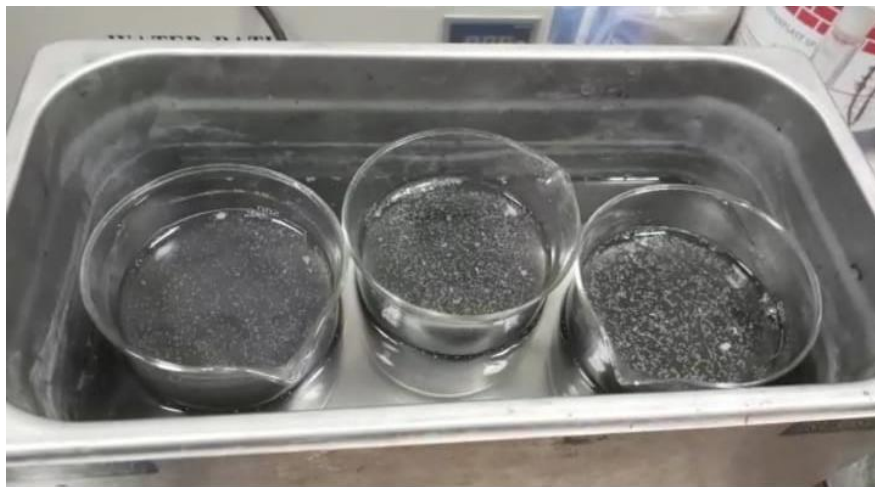
Figure 3: shows ultrasonication bath being used for dispersion of GNPs.
