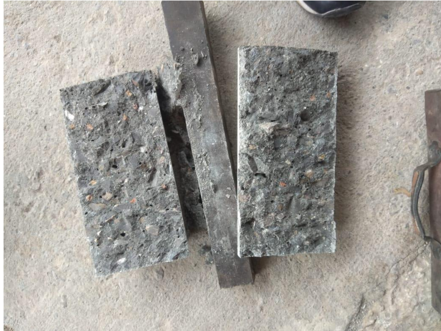
Figure 12: shows sample after split tensile test.
