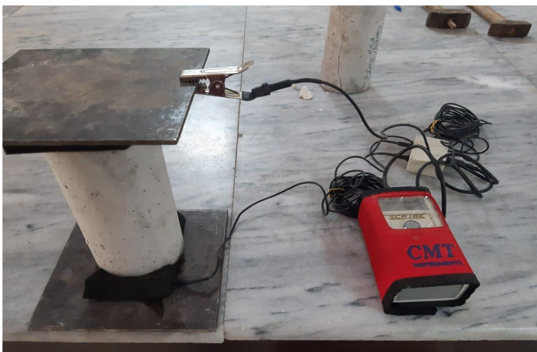
Figure 18: shows electrical resistivity test apparatus and specimen
