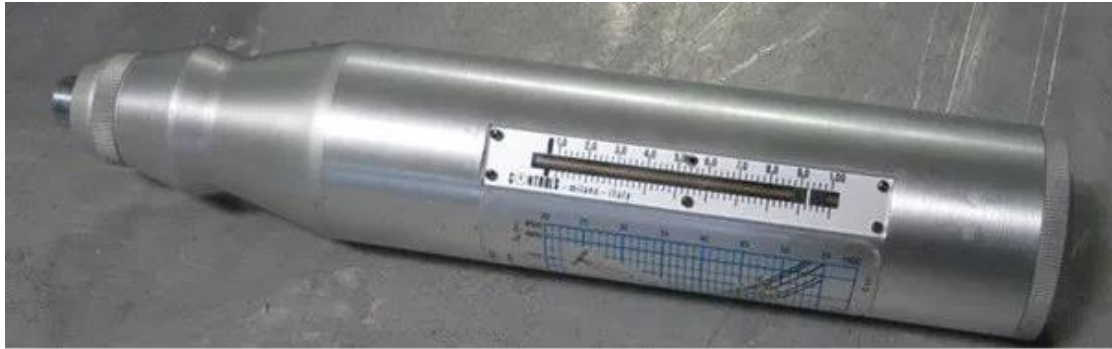
Figure 21: shows the rebound hammer
