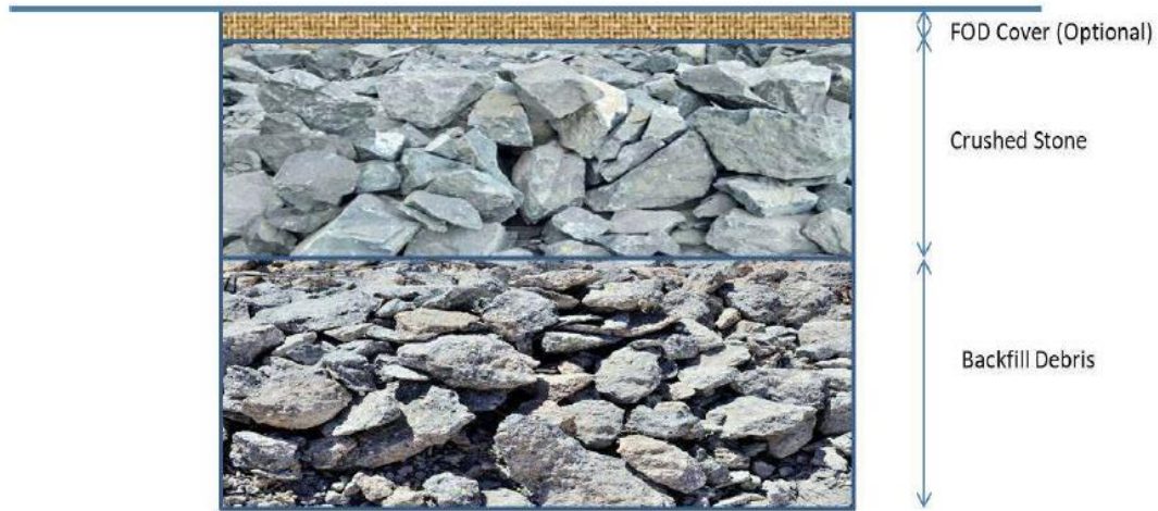
Figure 2.5: RRR by crushed stone
