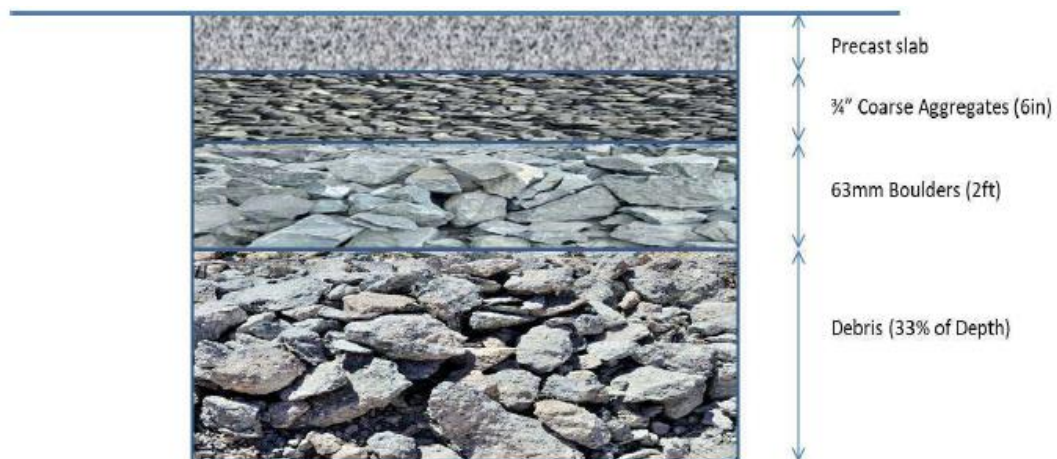
Figure 2.2: RRR by Concrete Slab
