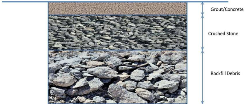
Figure 2.1: RRR by grouting or placing concrete.
