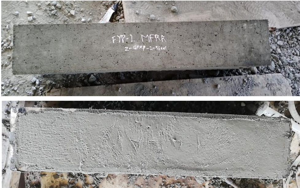
Figure 3.8 Casted Concrete Beam of 750mm
