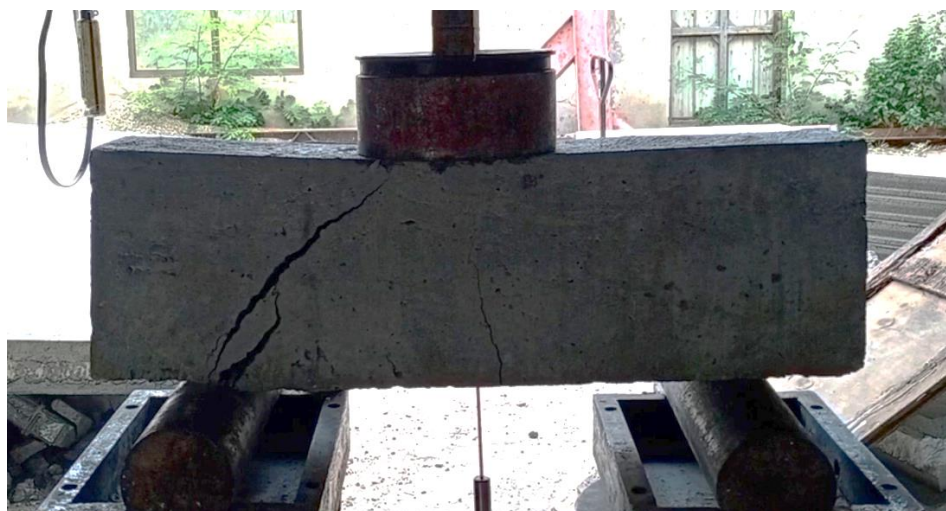
Figure 4.5 Failure of GFRP reinforce 750 mm span beam
