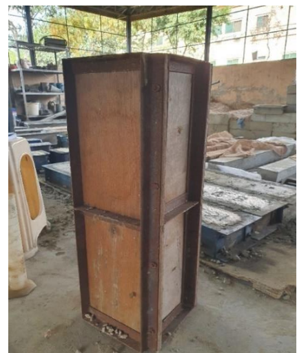
Figure 1 mold used for initial casting.
