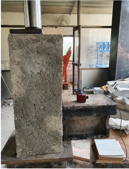
Figure 12 Retrofitted Specimen with surface preparation Testing
