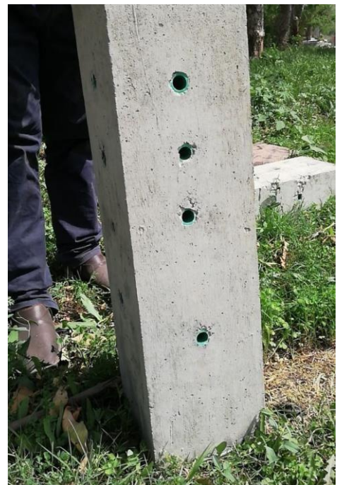
Figure 2 Specimen to be Retrofitted
