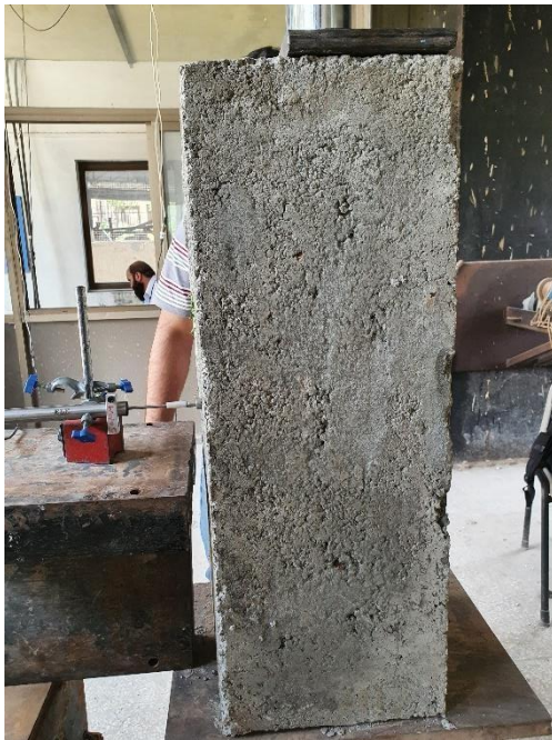
Figure-10 Retrofitted Specimen without surface preparation Testing
