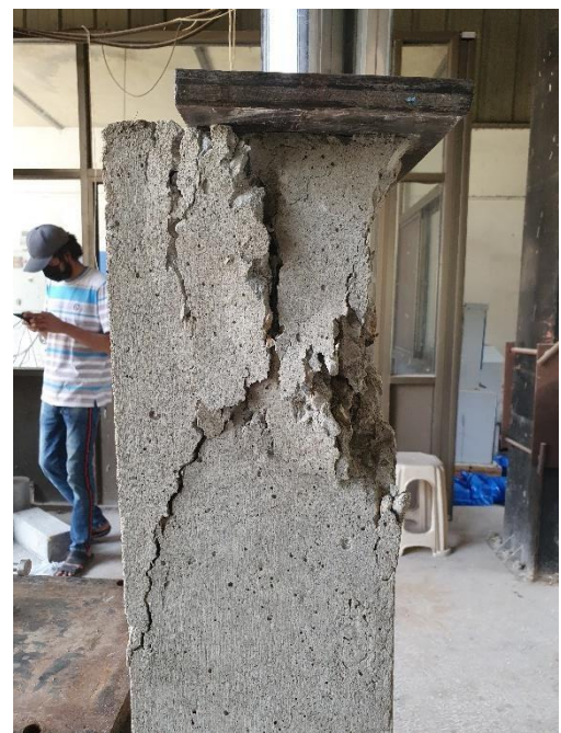
Figure 9 Base Specimen Failure
