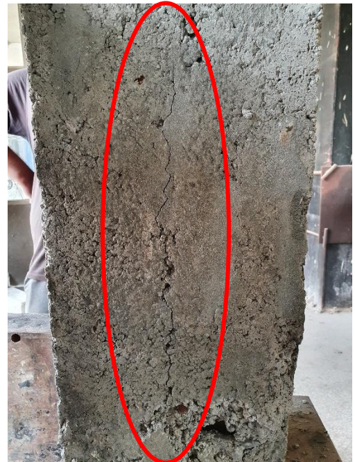
Figure-11 Retrofitted Specimen without surface preparation Cracking.
