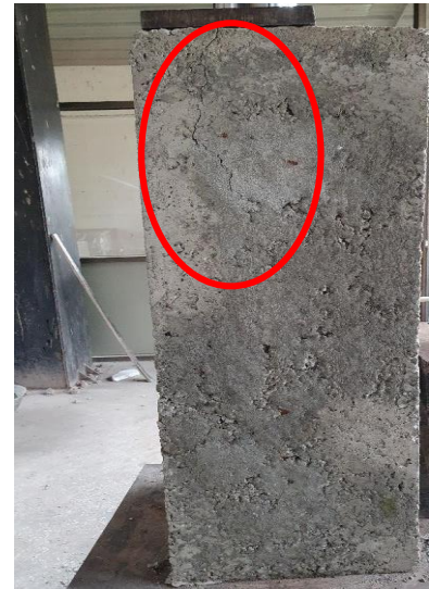
Figure 13 Retrofitted Specimen with surface preparation Cracking.
