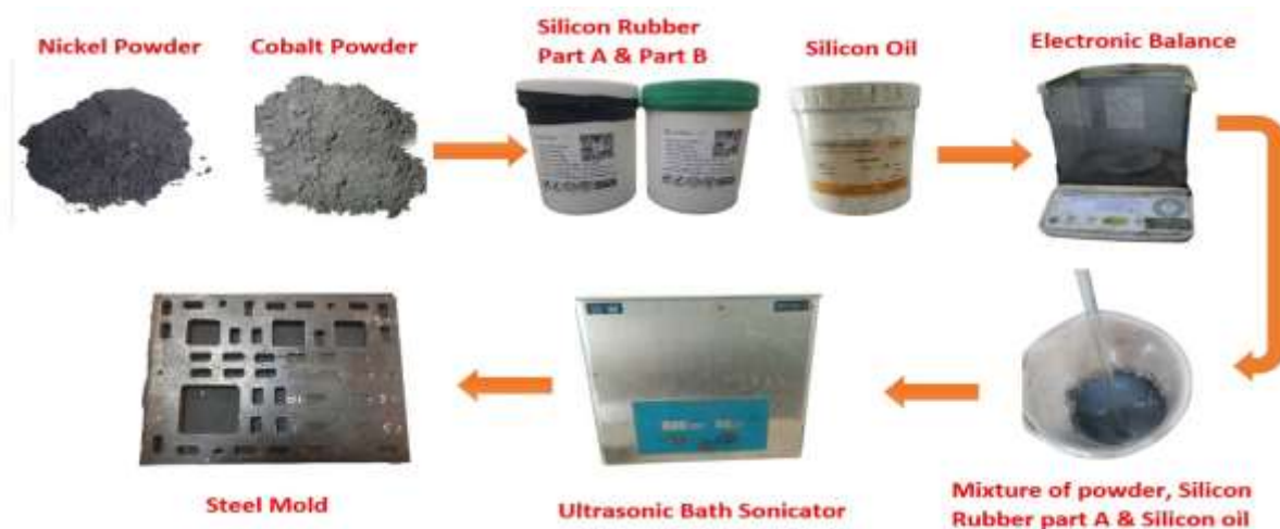
Figure 4. 12: Steps for casting of magnetorheological elastomers
