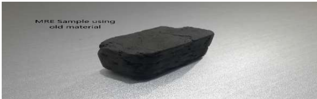
Figure 3. 1: MRE Sample at 15% Filler Content
