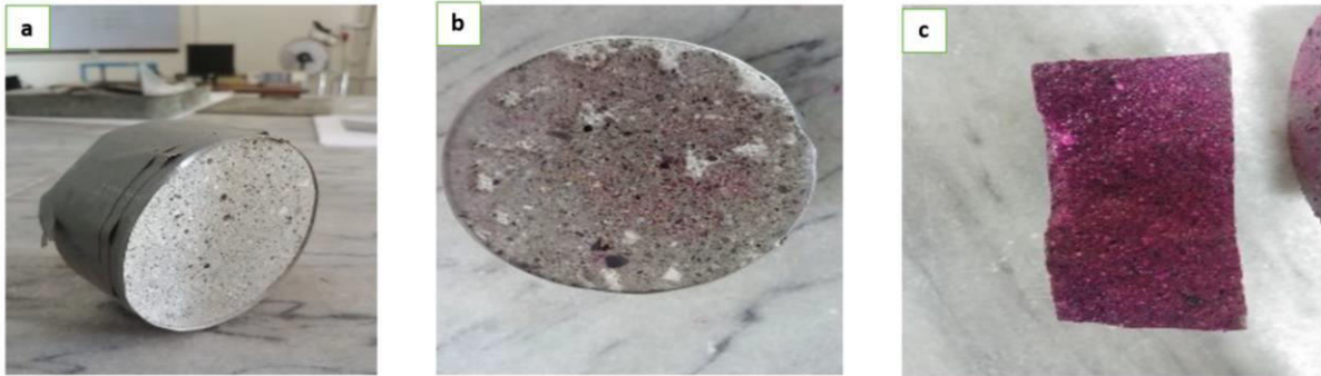
Figure 5.5.1: (a) Specimen Before Testing (b) Surface Carbonation (c) Specimen Split and check for carbonation
