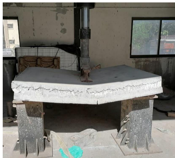
Figure 4.2.3: Test Setup for three-point bending test of slab panel
