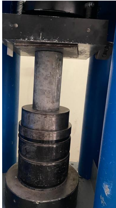
Figure 15: Compressive Strength Test Cylinder in UTM
