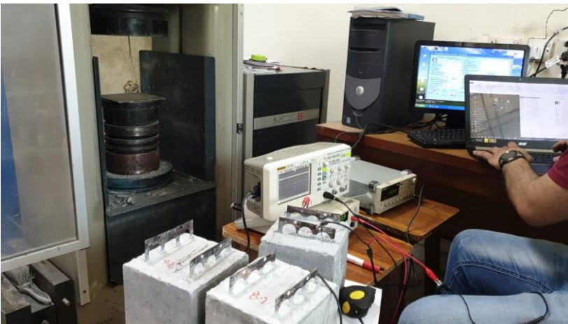
Figure 19: Piezoresistive Testing apparatus Setup
