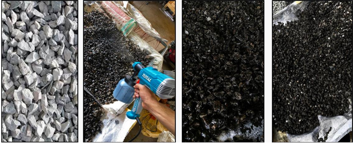
Figure 9: Coarse aggregate before and after coating
