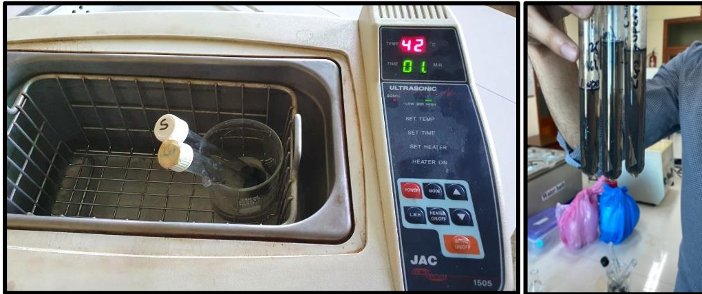
Figure 11: Sonication in Progress, Glass test tubes having different proportions
