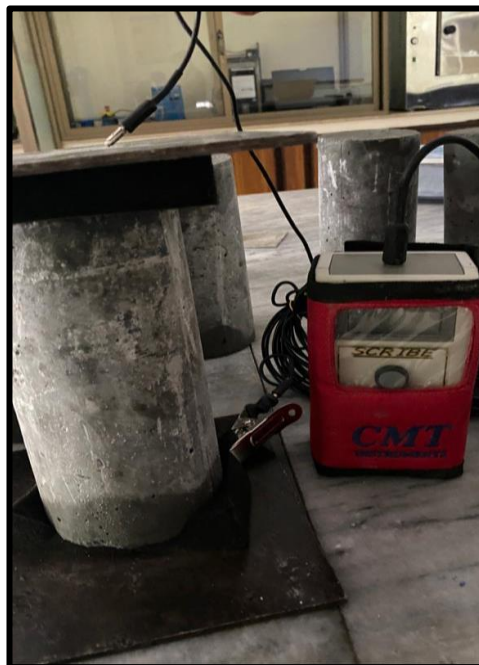
Figure 17: Bulk Resistivity Test
