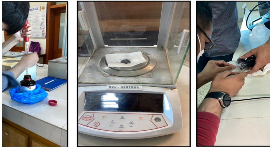
Figure 7: Preparation of CNP based ink
