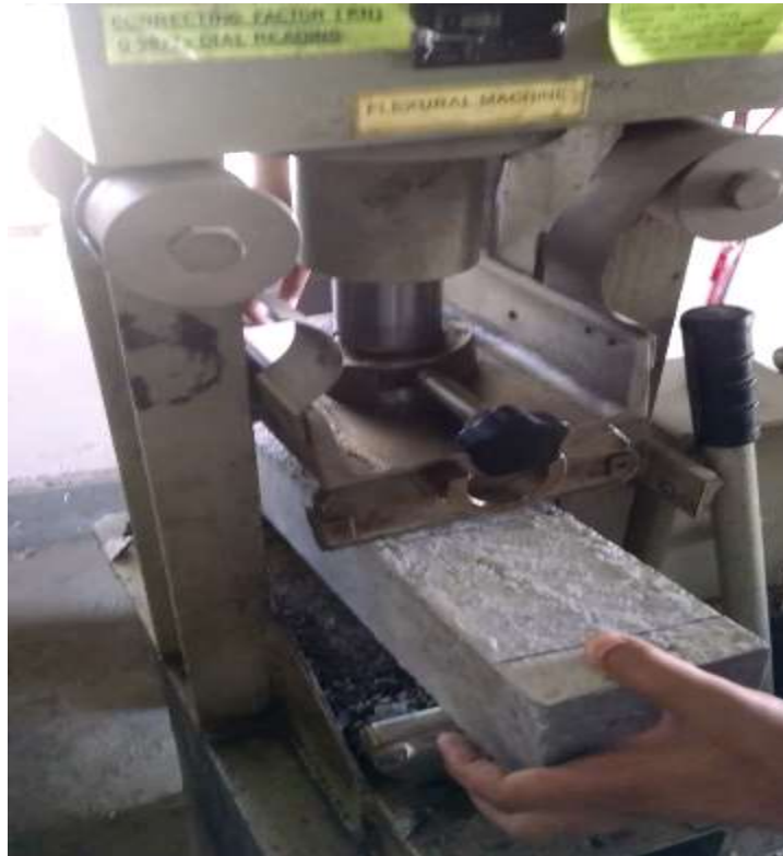
Figure 12. Testing of sample for flexural strength
