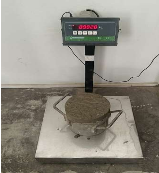
Figure 6. Measurement of fresh density of concrete.
