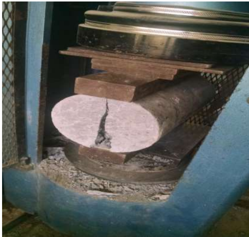
Figure 10. Testing of a sample for split tensile strength
