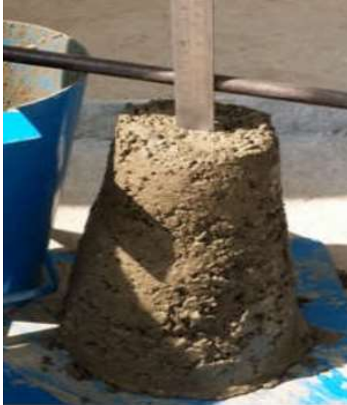
Figure 4. Measurement of slump of a concrete mixture
