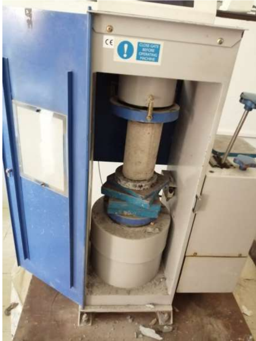
Figure 7. Testing of Compressive strength of a concrete sample
