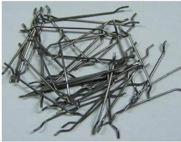
Figure 6: Hooked Steel Fibres
