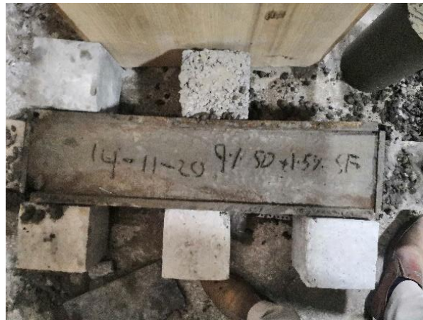
Figure 10: Casting of Beam Prism
