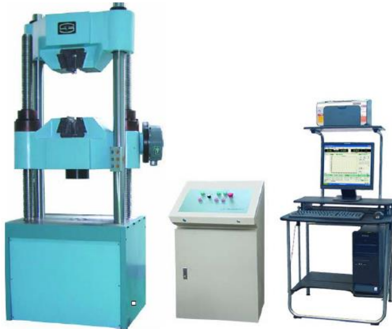
Figure 12: Universal Testing Machine
