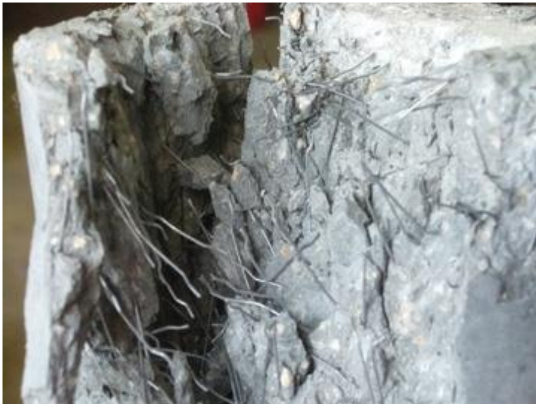
Figure 3: Steel Fibre Reinforced Concrete after Failure [9]
