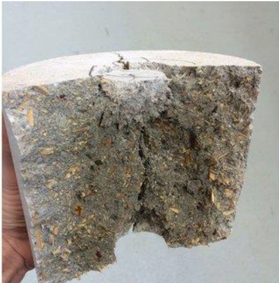
Figure 2: Saw dust modified concrete [33]
