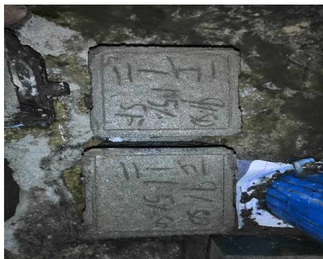
Figure 8: Casting of Cubes
