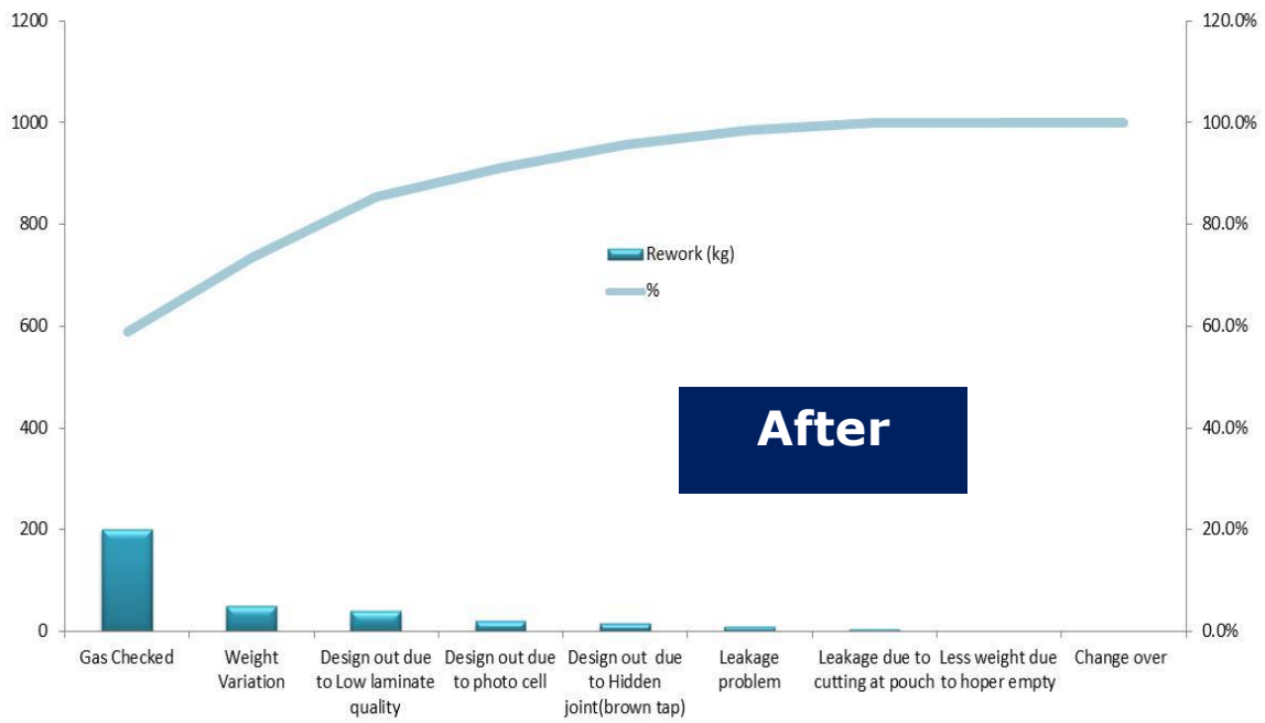
Figure 45 Pareto chart of losses causes after DMAIC showing significant improvement
