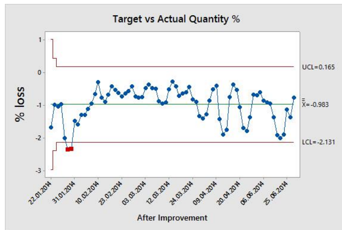
Figure 42 control chart for losses after DMAIC
