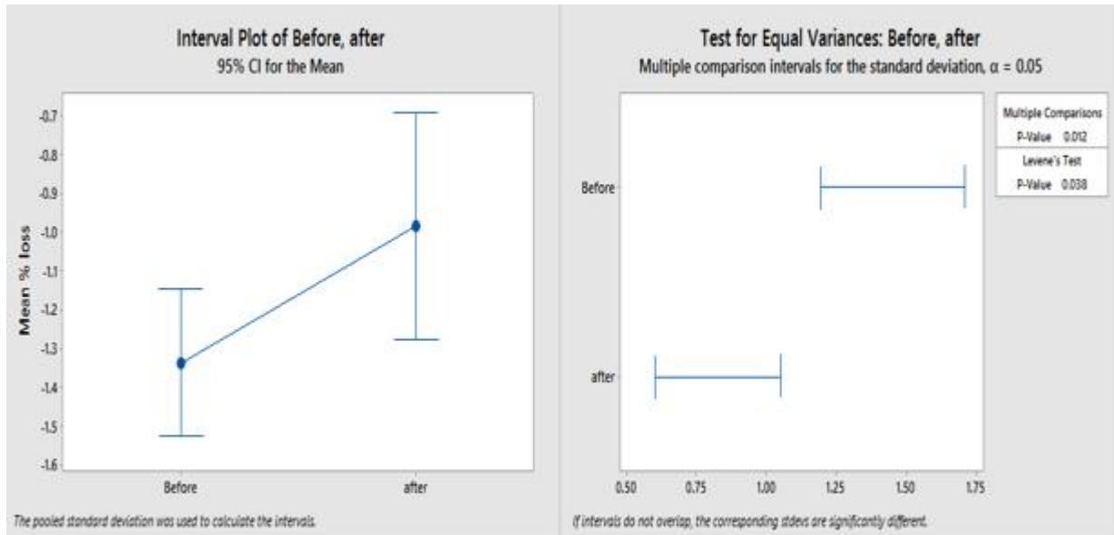
Figure 43 Comparison of mean losses before and after DMAIC using MINI_TAB
