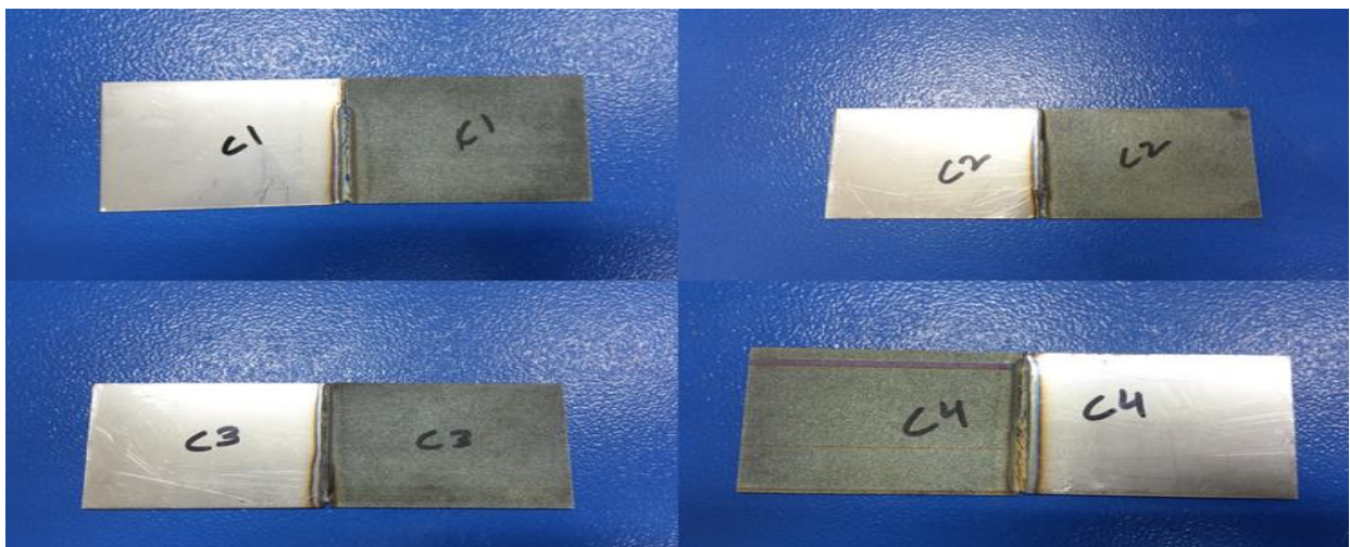
Figure 3.12: Laser welding of SS-Ti with Copper as filler
