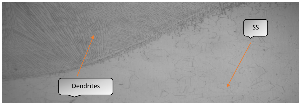
Figure 4.13: Interface between SS and weld zone.
