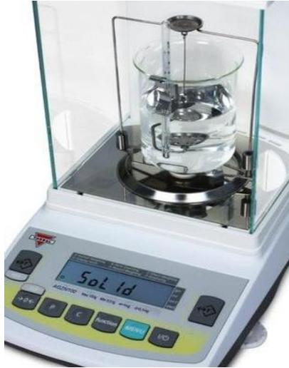
Figure 3.5: Density Measurement apparatus
