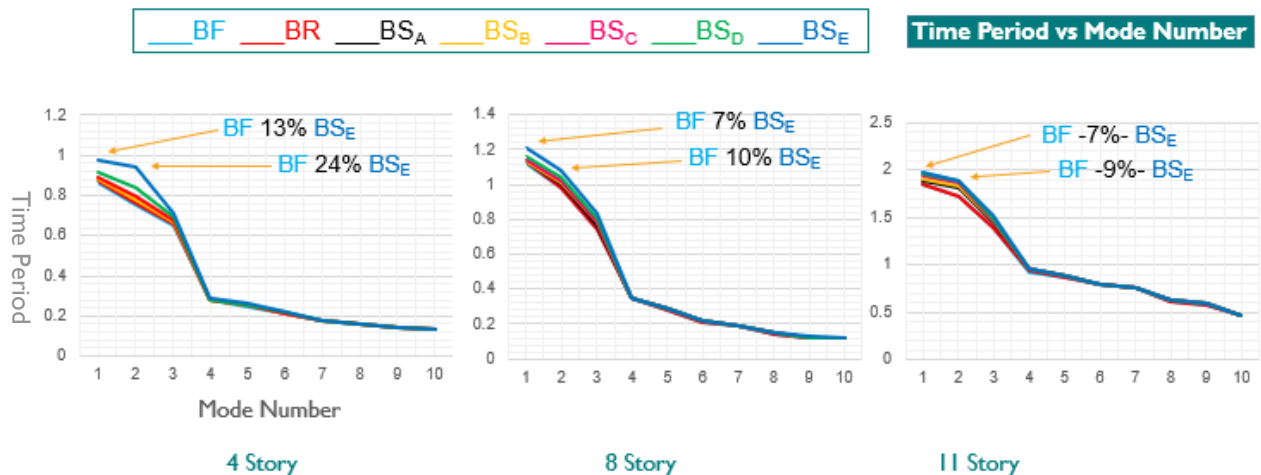
Figure 4-2: Fundamental time period variation of buildings
