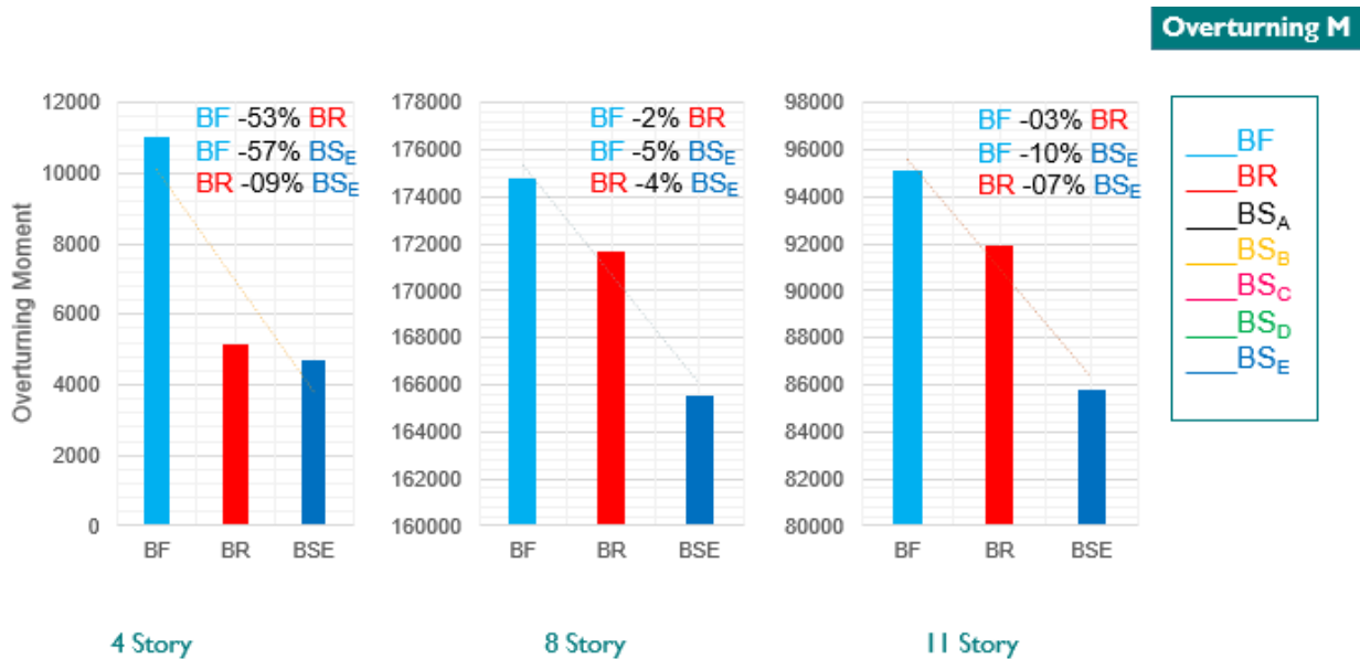
Figure 4-10: Overturning moments comparison for BF, BR and BS A
