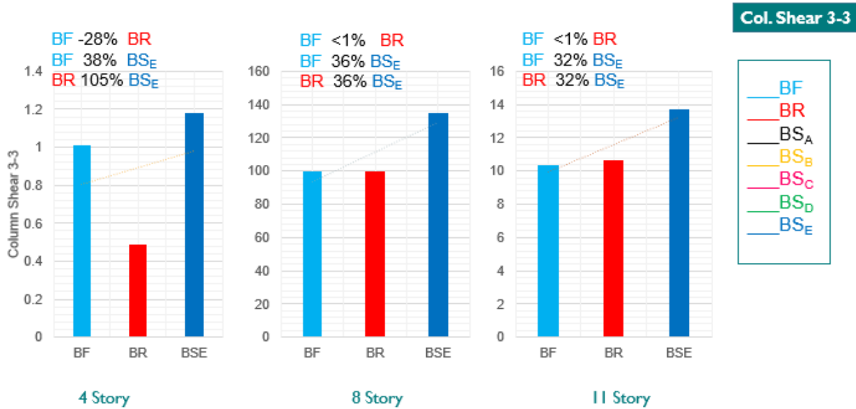
Figure 4-17: Column shear in 3-3 direction comparison of BF, BR and BSA
