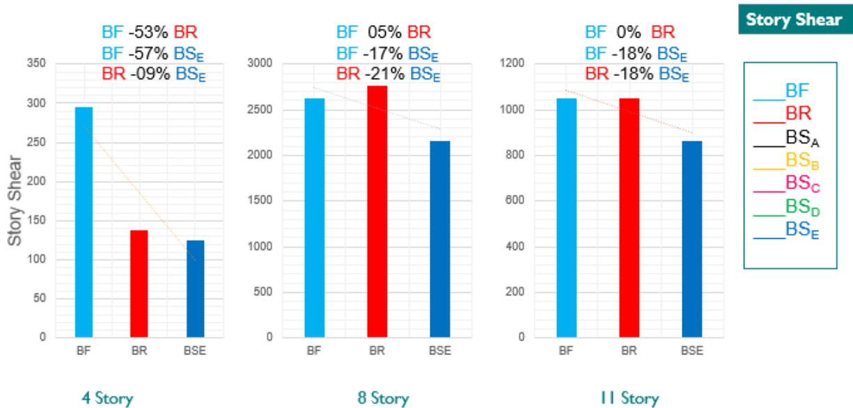
Figure 4-8: Maximum story shear comparison for BF, BR and BS A
