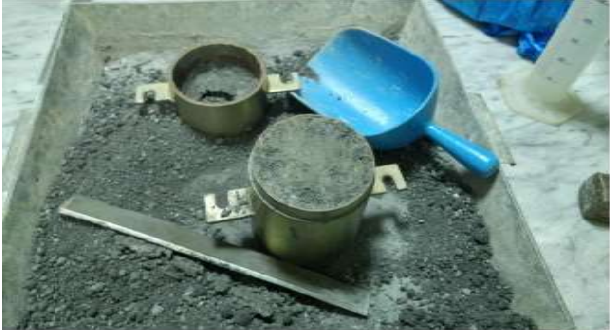
Figure 3.7. Standard proctor test in progress
