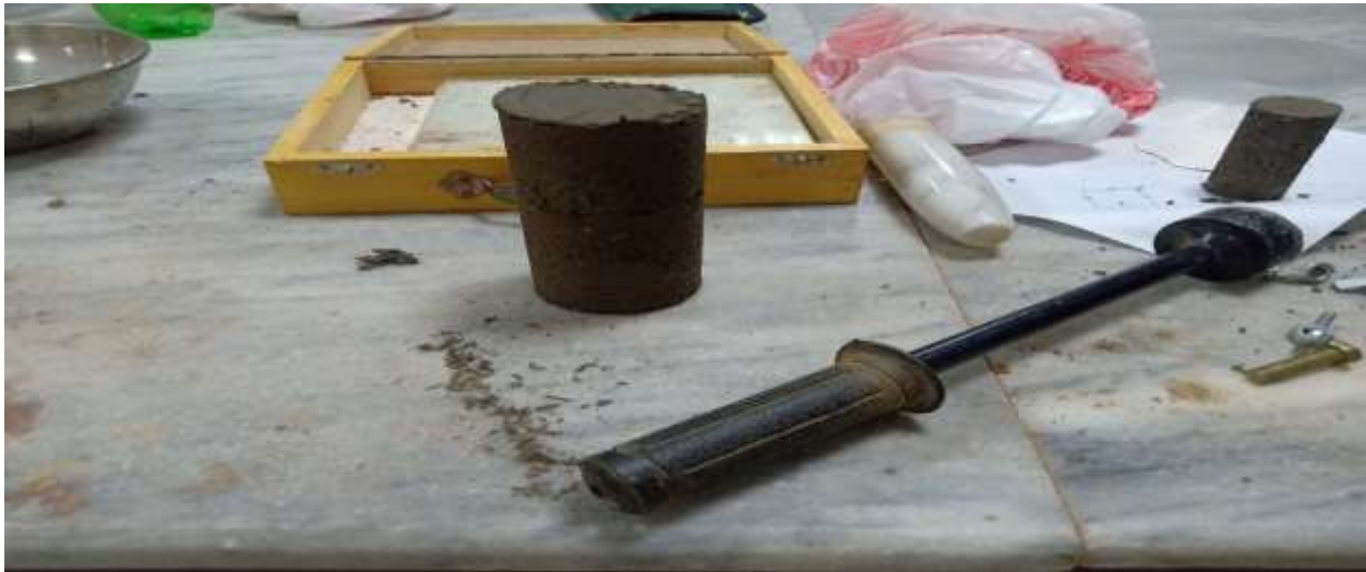
Figure 3.9. Sample preparation for unconfined compressive strength test
