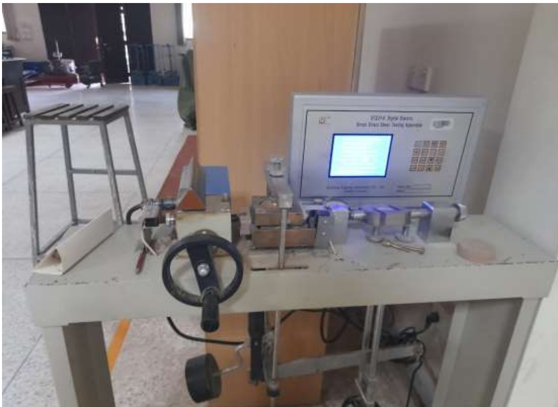
Figure 3.8. Direct shear test in progress
