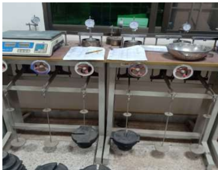
Figure 3. 11. One dimensional consolidation test in progress
