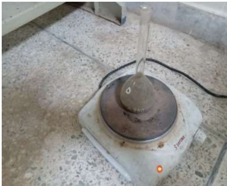
Figure 3.6. Specific gravity test in progress
