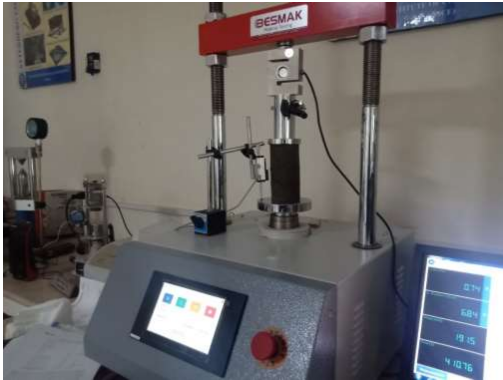
Figure 3.10. Unconfined compression test in progress
