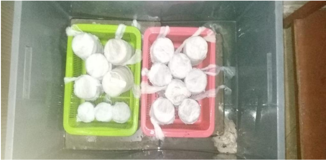
Figure 3.15: Saturation process is in progress
