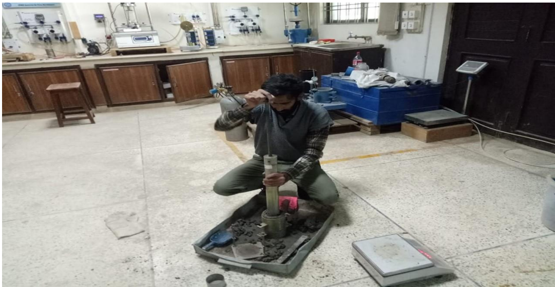
Figure 3.7: Standard Proctor test performed in the laboratory
