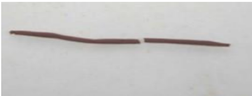
Figure 3.4: Appearance of thread after plastic limit test
