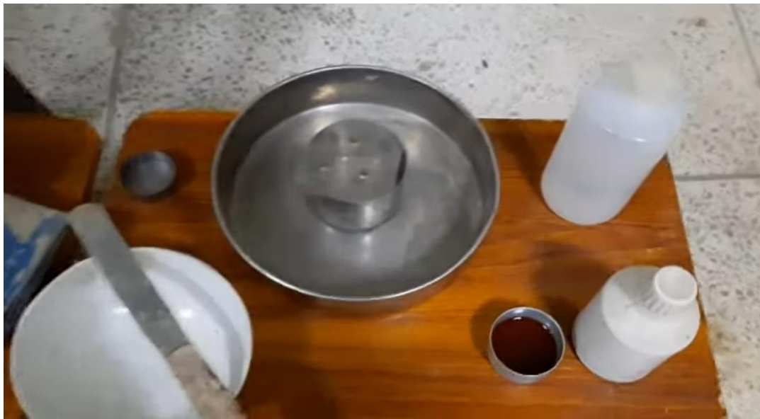
Figure 3.5: Shrinkage limit arrangement in the laboratory
