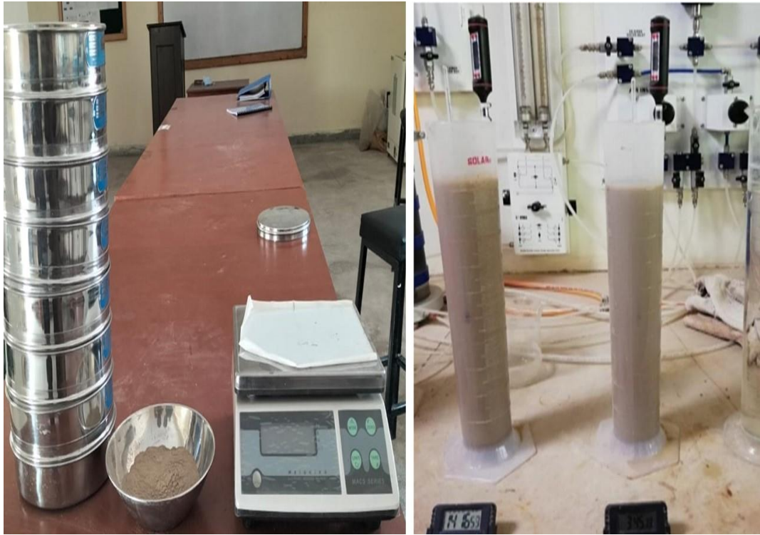
Figure 3.2: Scheme of sieve analysis and hydrometer analysis in the laboratory
