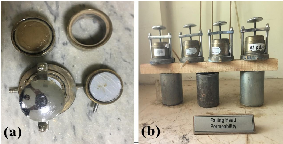
Figure 3.10: Pictorial views of hydraulic conductivity tests in the laboratory
