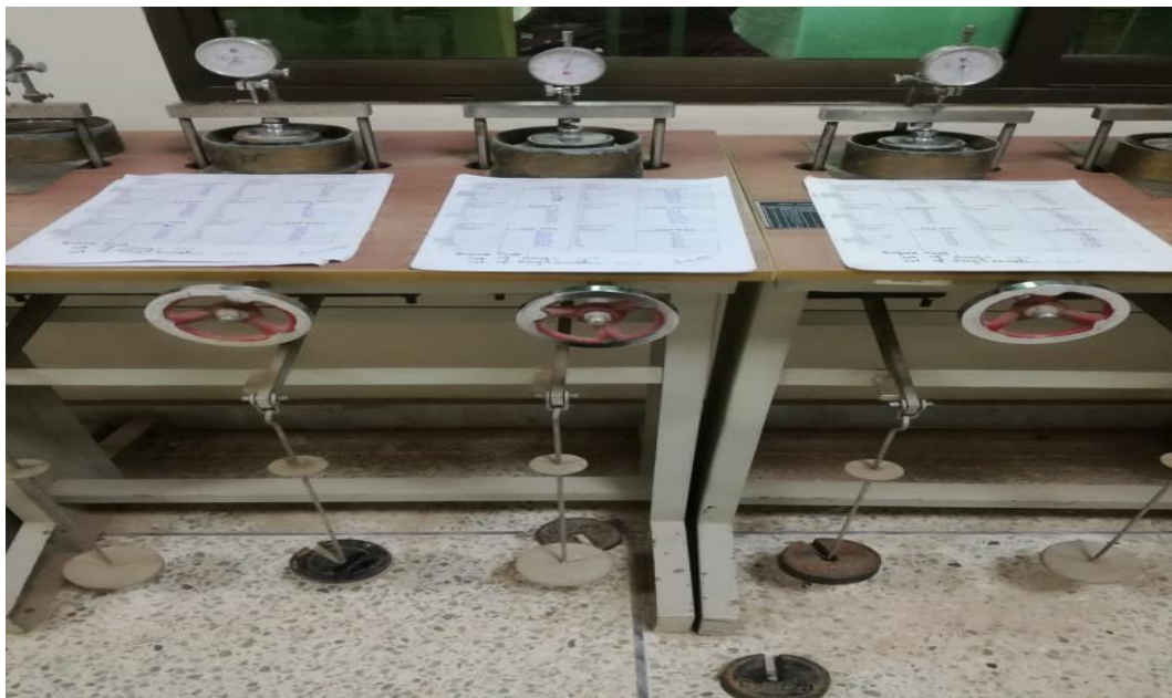
Figure 3. 8: Consolidation test progression in unsaturated condition
