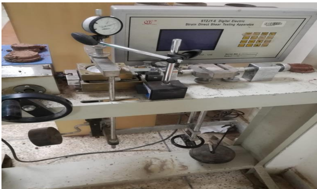
Figure 3. 5: Direct shear test arrangements in the laboratory
