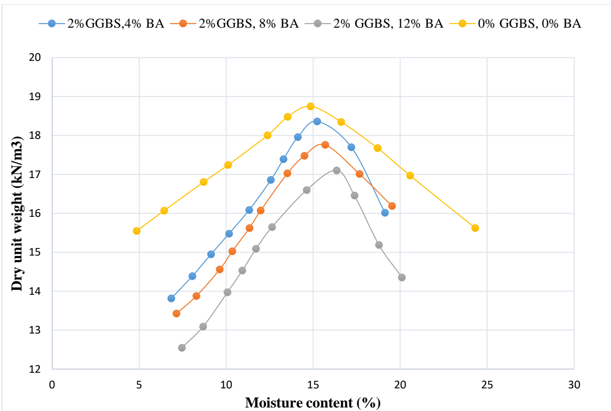
Figure 4. 5: Compaction curves of treated collapsible soil
