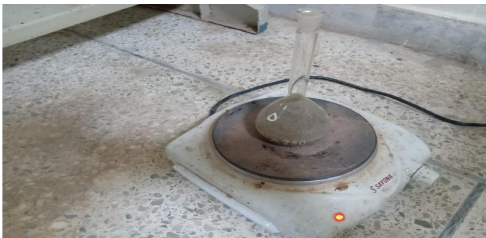
Figure 3. 3: Specific gravity test progress in the laboratory
