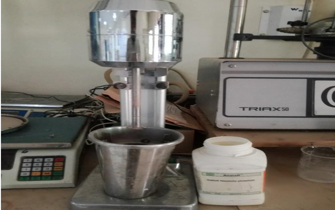
Figure 3. 1: Apparatus for hydrometer analysis
