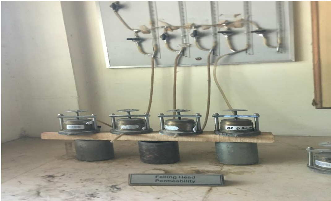
Figure 3. 6: Falling head method for determination of hydraulic conductivity of fine grained soil
