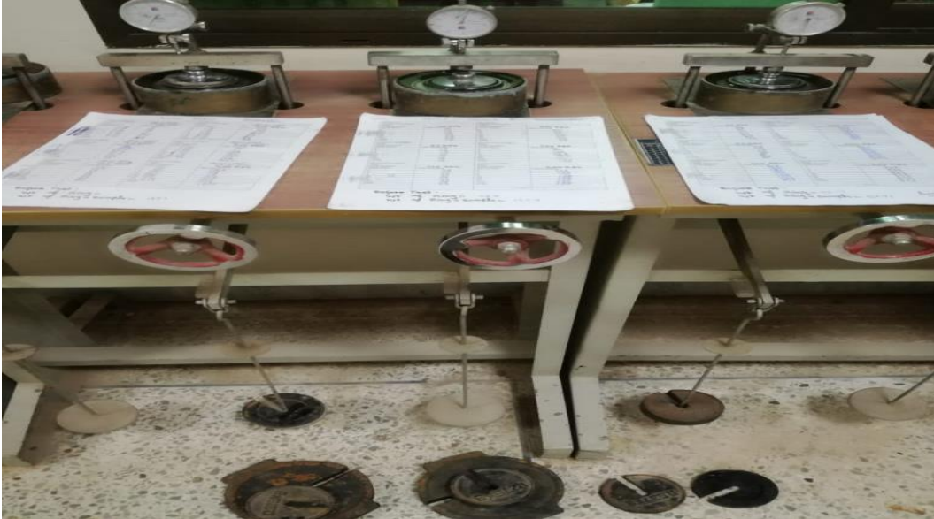
Figure 3. 7: Consolidation test in saturated condition
