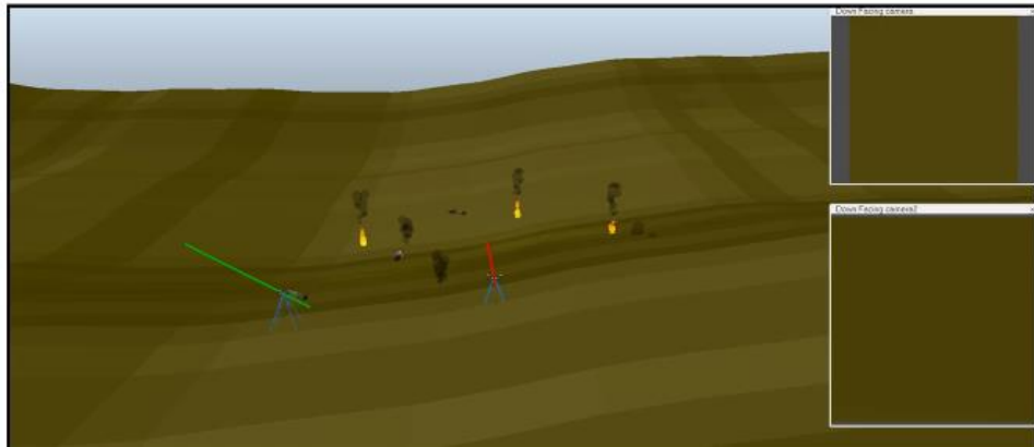
Figure 22: Multiagent UAVs parallel track search simulation in VREP
