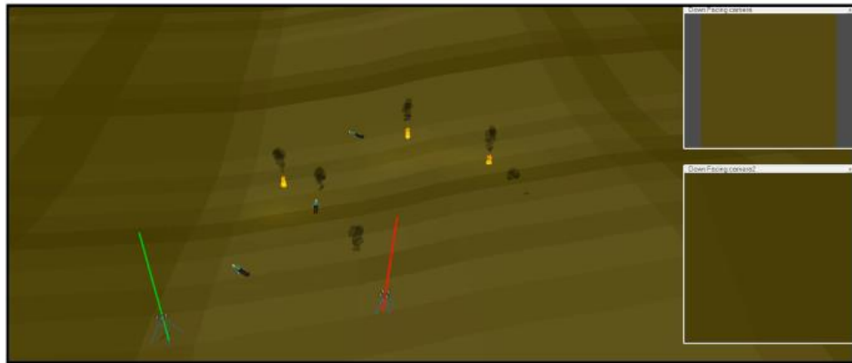
Figure 24: Multiagent UAVs hybrid search simulation in VREP
