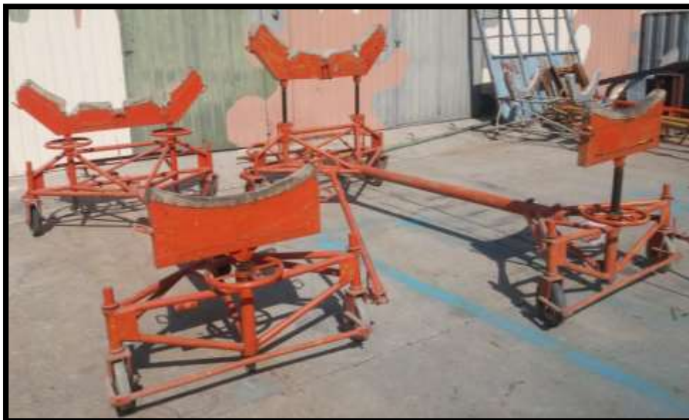
Figure 4.11: UAV Transportation Trolley
