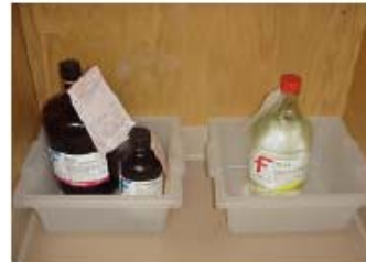
Proper Hazardous Waste Storage. Hazardous waste is labeled, segregated by compatibility, stored in secondary containment, and in an isolated area.
