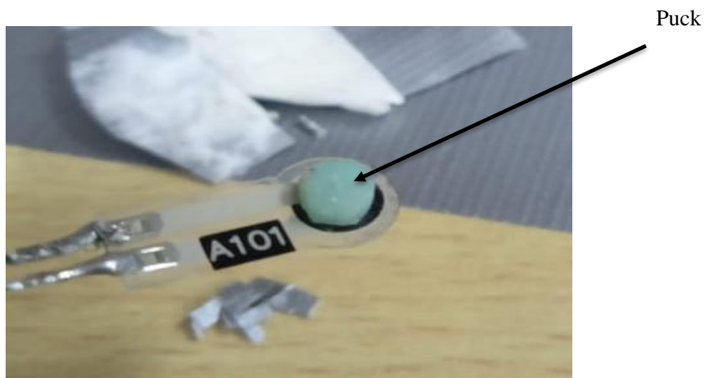
Figure 17: Puck is placed on above the sensor
