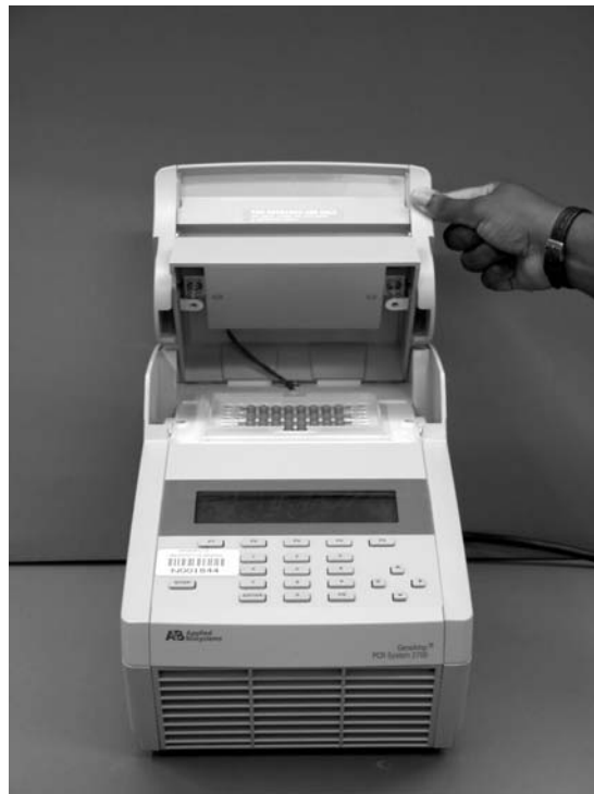
Figure 24-2 A thermal cycler that is used to conduct PCR using defined temperatures for specific time intervals. (Photo courtesy K.L. Josephson.)
