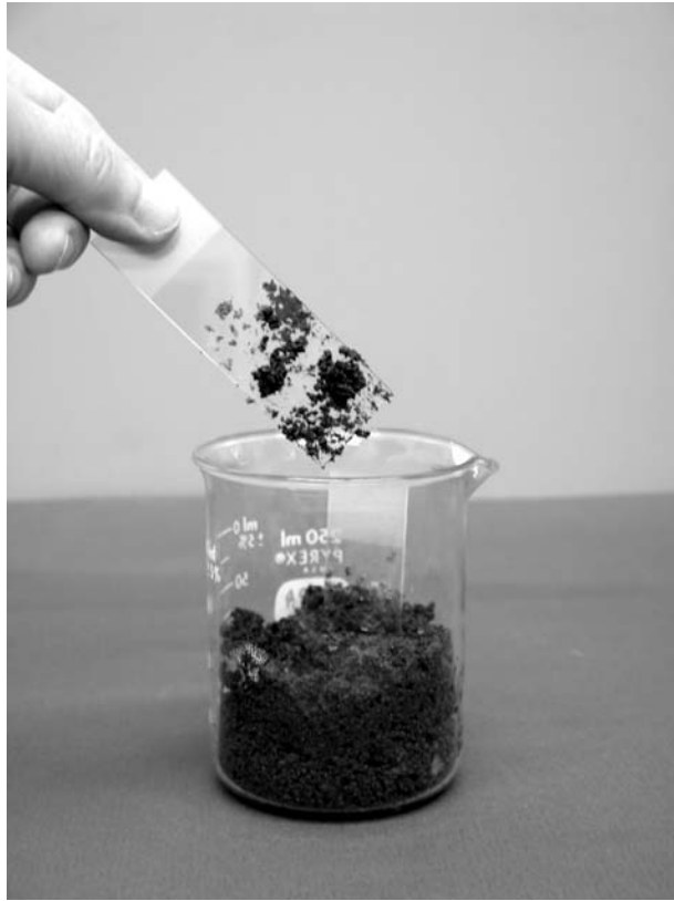
Figure 3-6 Example of how the slide plus accompanying soil should look following removal of the slide from the soil (Photo courtesy K.L. Josephson).
