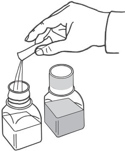
Figure 17-3 A tube of Colilert ® reagent is being added to a water sample in a sterile, non-fluorescent container. The container to the right has turned yellow after incubation at 35 \pm 5^\circ\text{C} for 24–28 h, thus testing positive for total coliforms.
